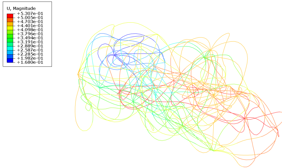
Figure 4.23. Hexakis icosahedron load case 3 deformed shape
