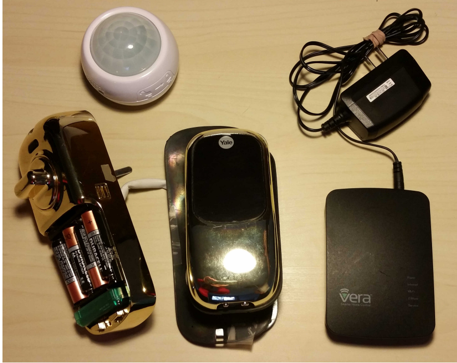
Figure 36. Devices used for the study are the Yale door lock (lower-left), Aeon Multi-sensor4 (upper-left), and MiCasa Verde-Edge controller (right).
