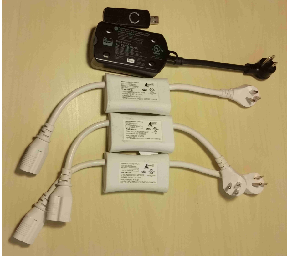
Figure 62. Devices used in the network under study. From top to bottom, this includes an Aeon USB ZStick2, a GE Outdoor Switch, and three Aeon Appliance Switches.
