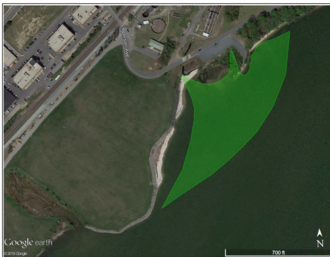
Figure 4. Approximate extent of TLC in the Quantico Embayment. The cap area encompasses sediment with surface sediment DDX concentrations greater than or equal to 200 µg/kg (Adapted from Battelle 2008).
