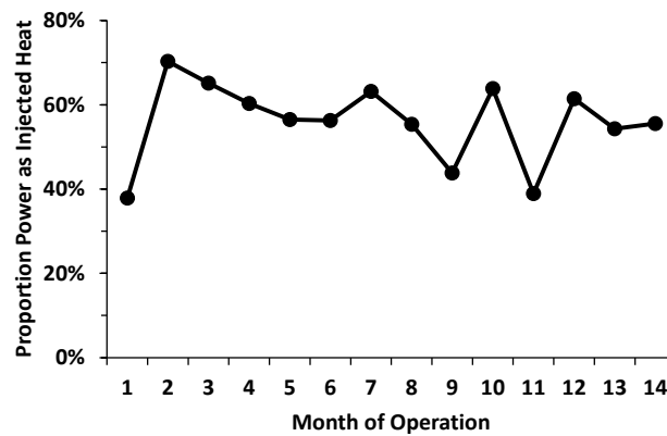
Figure 5.7.20. Proportion of Estimated Power Consumption as Injected Heat During XSVE Operation.
