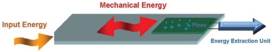
Fig. 3.3 Schematic diagram of a vibration energy harvesting system
