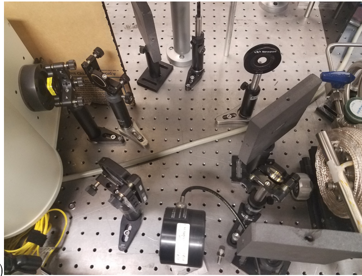
Figure 9. Close up of the collection optics. a) Heat pipe pumped from the right, left is a fiber looking at a 600 grit silver diffuser plate that goes to our spectrometer in the 300-850 nm range; with the filter wheel set to move the diffuser plate, the laser light hits the collimator on the right that goes to our 900-2000 nm spectrometer. b) Heat pipe is pumped from the left, output hits a fused silica substrate high power mirror to filter out the pump and let 3000 nm light through; this light hits two gold mirrors and a 35 mm \text{CaF}_2 coupling lens to our 3000-5000 nm spectrometer.
