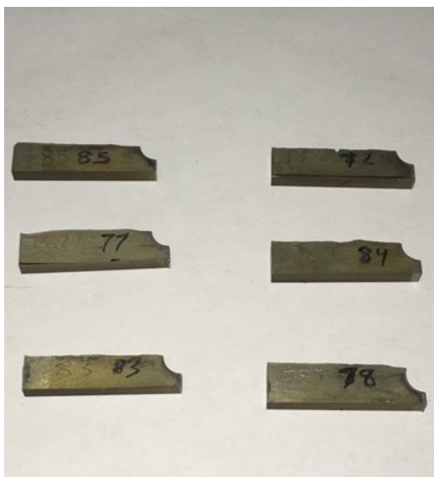
Figure 70. Cadmium coated specimens prepared for SEM analysis.
