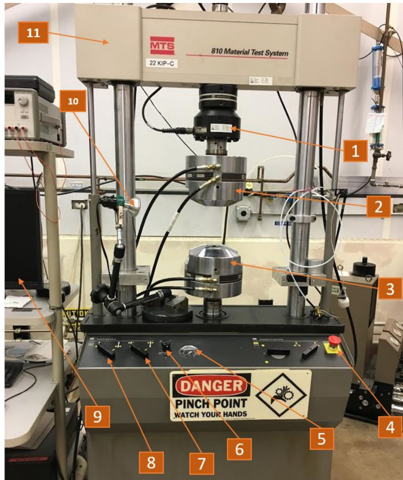
Figure 14. Test machine components: (1) load cell, (2) passive upper grip, (3) active lower grip, (4) emergency stop button, (5) grip pressure gauge, (6) grip pressure adjuster, (7) upper grip controller, (8) lower grip controller, (9) control system, (10) lamp (11) frame.
