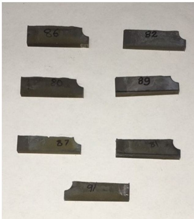
Figure 69. Zinc-Nickel coated specimens prepared for SEM analysis.
