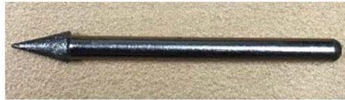
Figure 15. File used for scribe damage.
