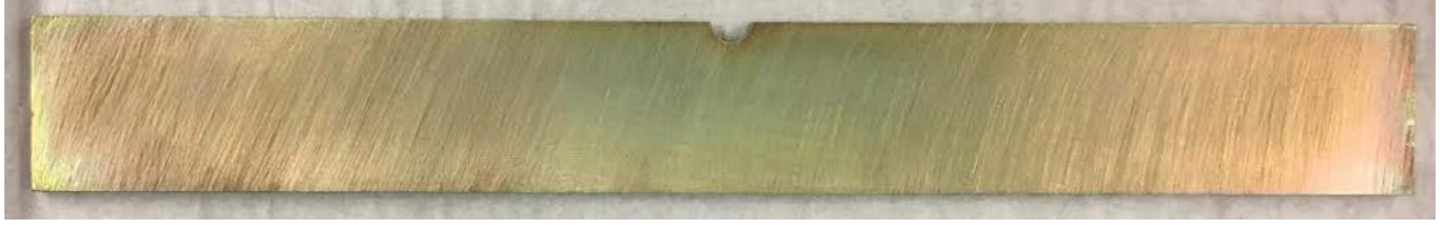
Figure 12. Specimen with Cadmium coating.
