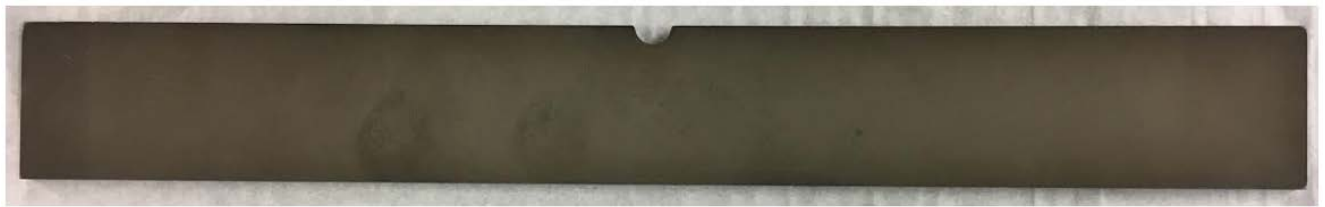
Figure 11. Specimen with Zinc-Nickel coating.
