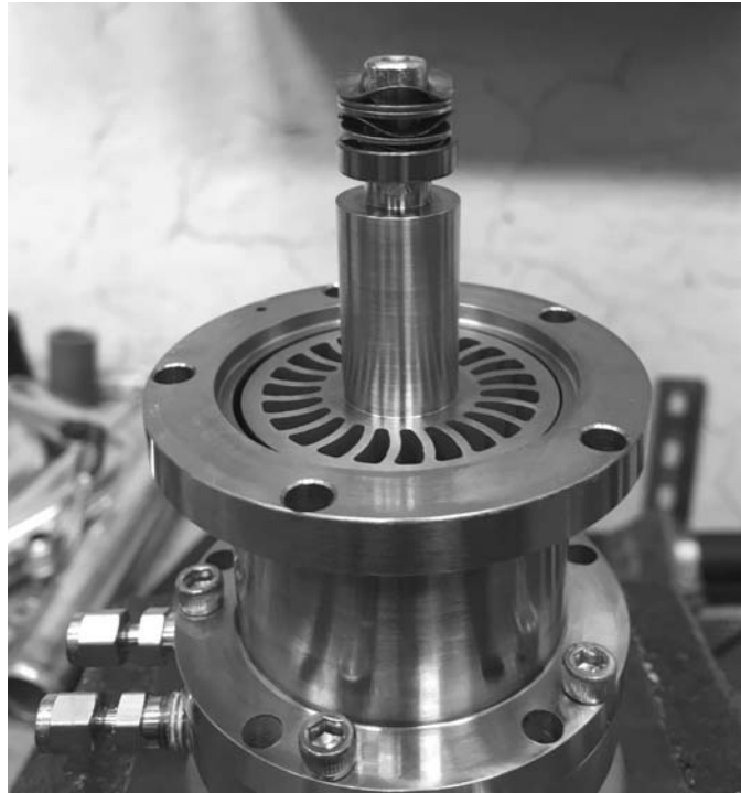
Figure 36 - Assembly Process with Washers and Bearing
