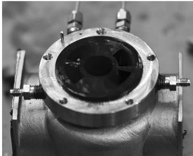
Figure 51 - Left Endwall Face with Carbon Deposits
