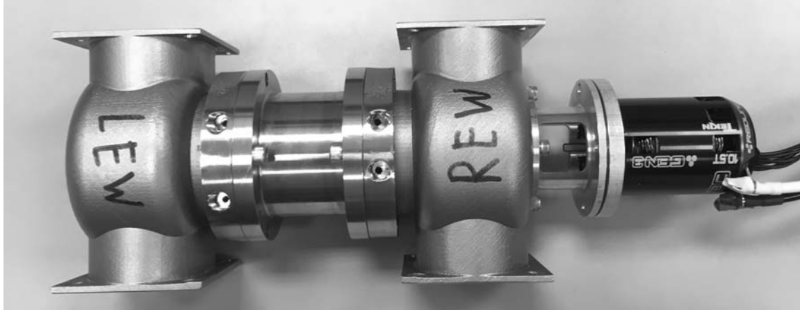
Figure 43 - Assembled Wave Rotor System with Motor
