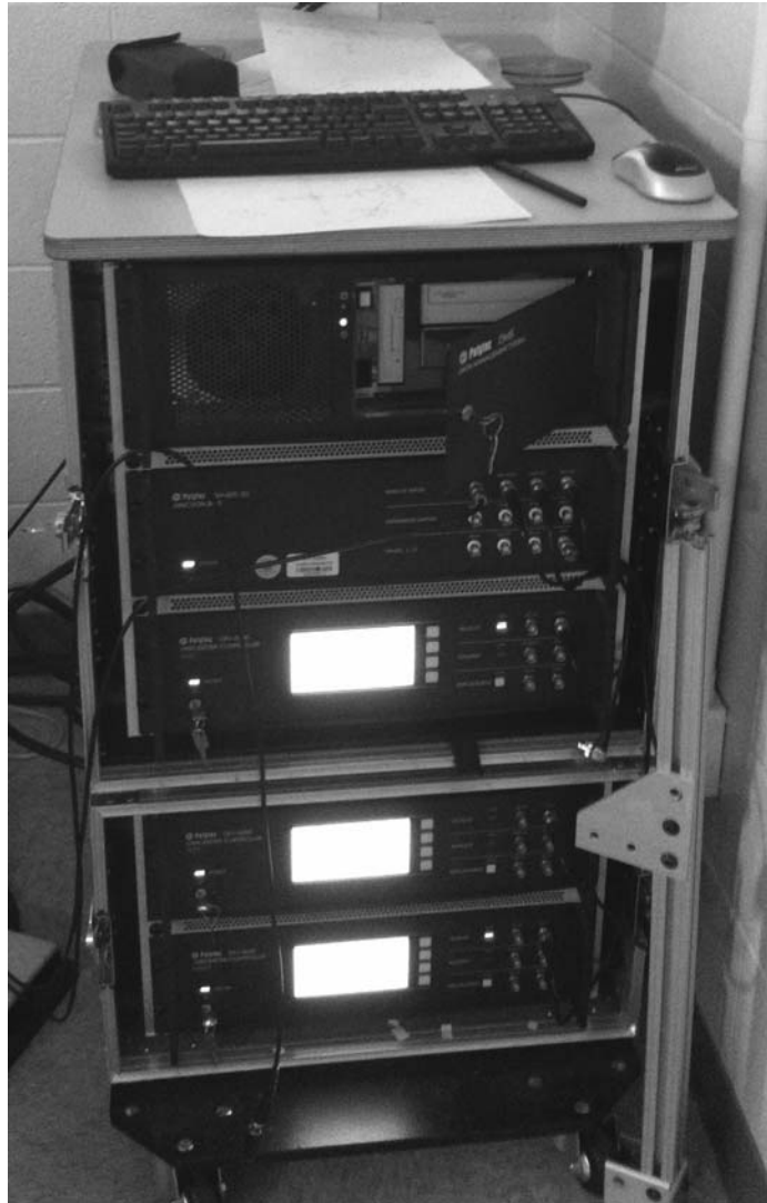
Figure 27. Polytec PSV-400-3D-M SLDV Equipment Rack.
