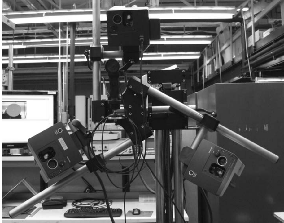
Figure 26. Polytec PSV-400-3D-M SLDV Scan Heads.
