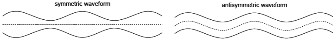
Figure 4. Symmetric and antisymmetric wave modes [60].
