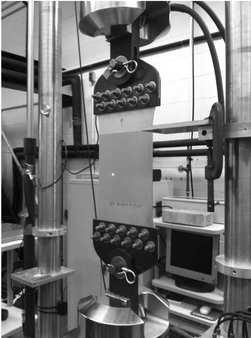
Figure 20. Example test specimen with retro-reflective film installed in MTS.
