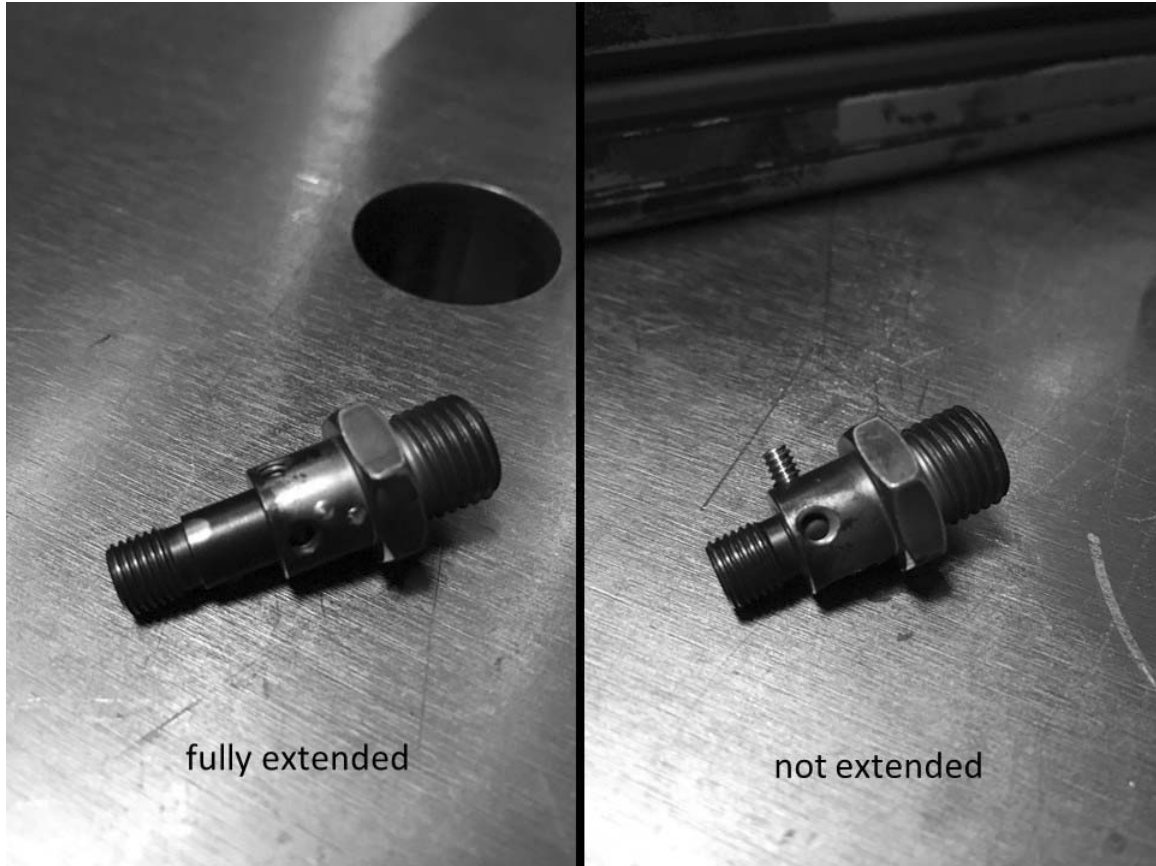
Figure 16. Collimating lens showing two adjustable positions used for FOV calculations.
