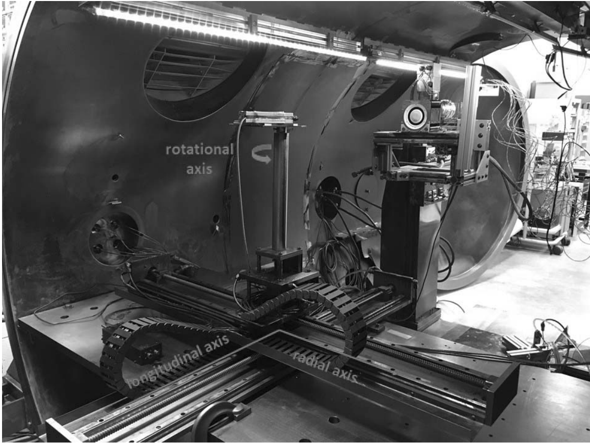
Figure 12. Translation stage installed in chamber upon which the fiber optic assembly is mounted showing axes of movement.
