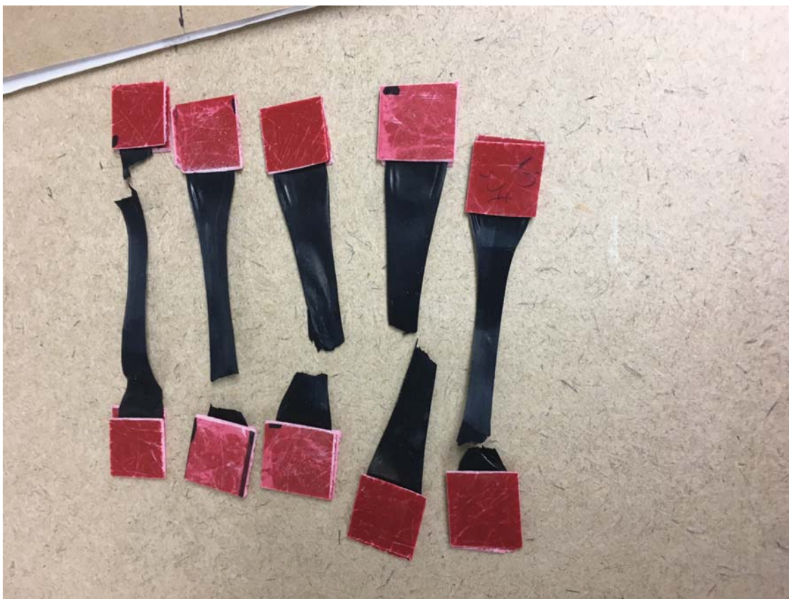
Figure 4.3. CNT Sheets after Tensile Testing
