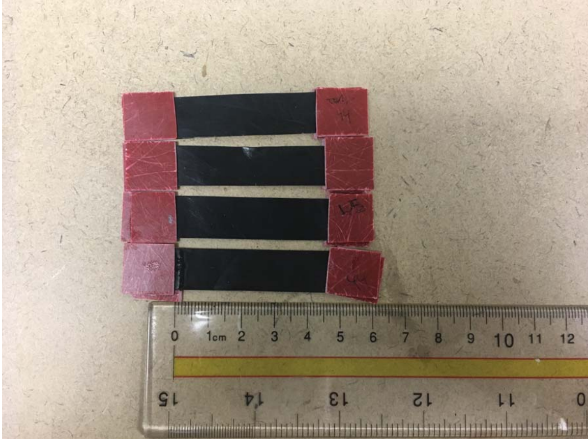
Figure 3.2. Untested specimens that have been mounted to the fiber glass.
