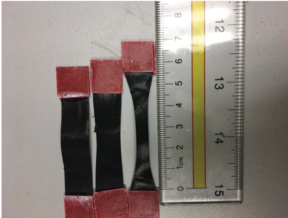
Figure 4.12. 3 Samples after creep tests at 10, 15, and 20 N applied load.
