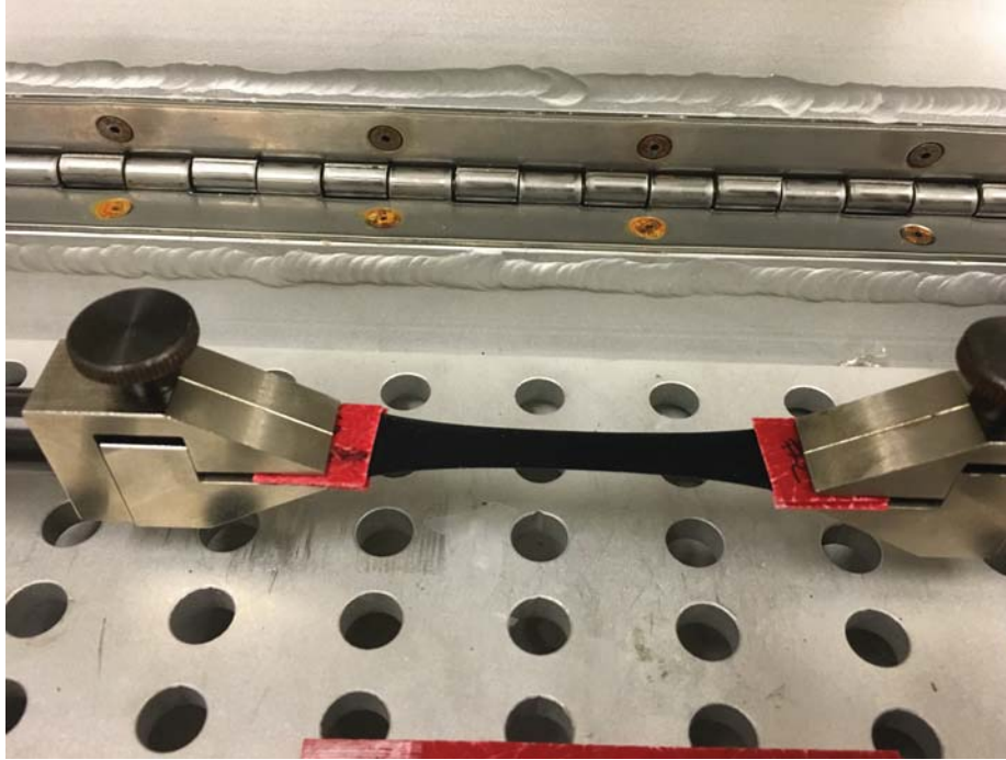
Figure 4.6. An example of a CNT sheet during creep testing at 15 N
