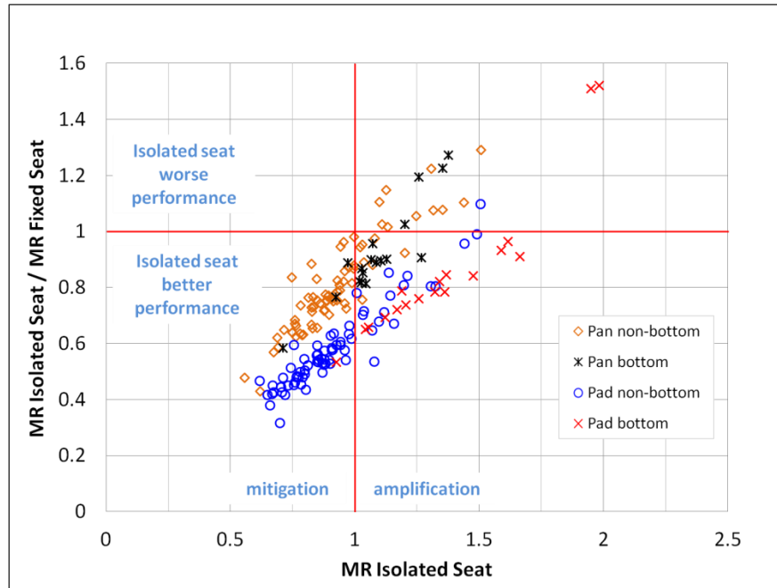
Figure G3. Ratio of Isolated and Fixed Pad and Pan MR Values
