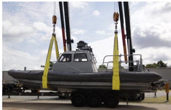
Figure 1. Figure Composite Hull 11m Cabin RIB
