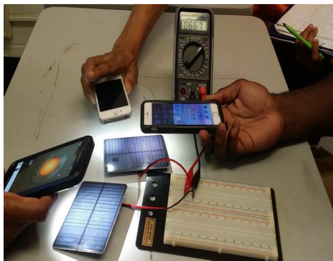
Figure 6. Solar cells connected in parallel 6.5 mA without load
