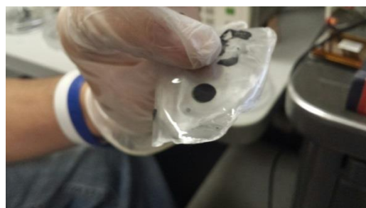
Figure 8. CNT Electrodes on PVA/Phosphorus Electrolyte
