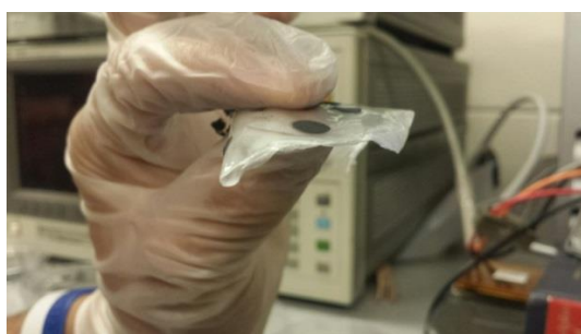
Figure 7. CNT Electrodes on PVA/Phosphorus Electrolyte
