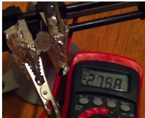
Figure 4. Piezoelectric crystal producing voltage
