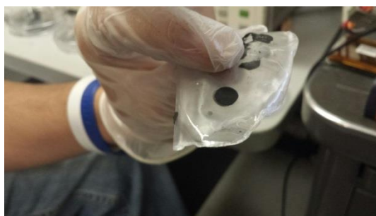
Figure 9. CNT Electrodes on PVA/Phosphorus Electrolyte
