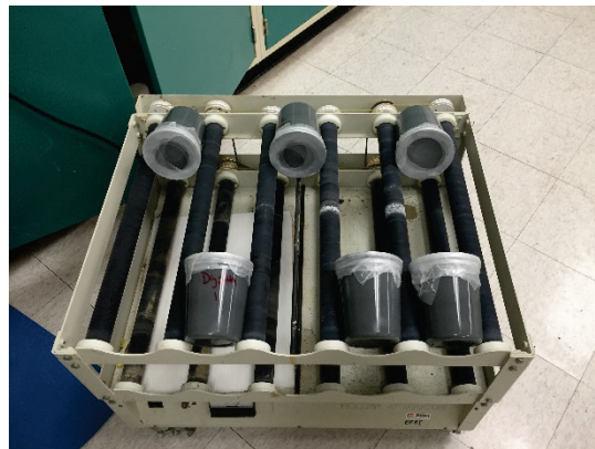
Figure 3. Roller mill mixing sediment.
