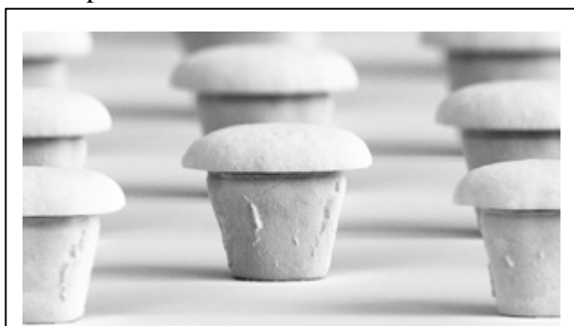
Figure 8. Electroplated electrodes with 10 \mu\text{m} wide pillars and rounded tops.
