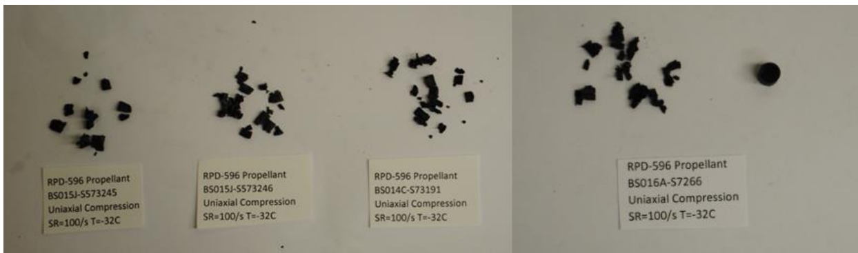
Figure 5 RPD-596 samples post-test at -32°C and an un-deformed grain on the right
