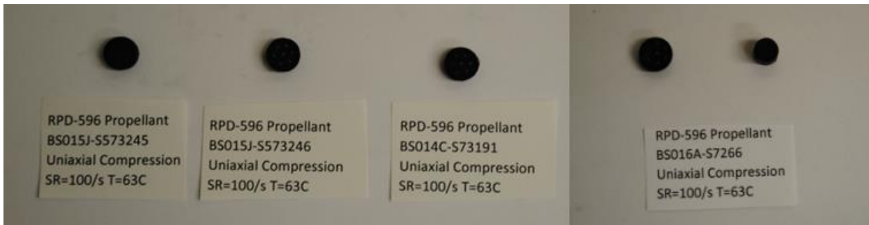
Figure 3 RPD-596 samples post-test at 63°C and an undeformed grain on the right
