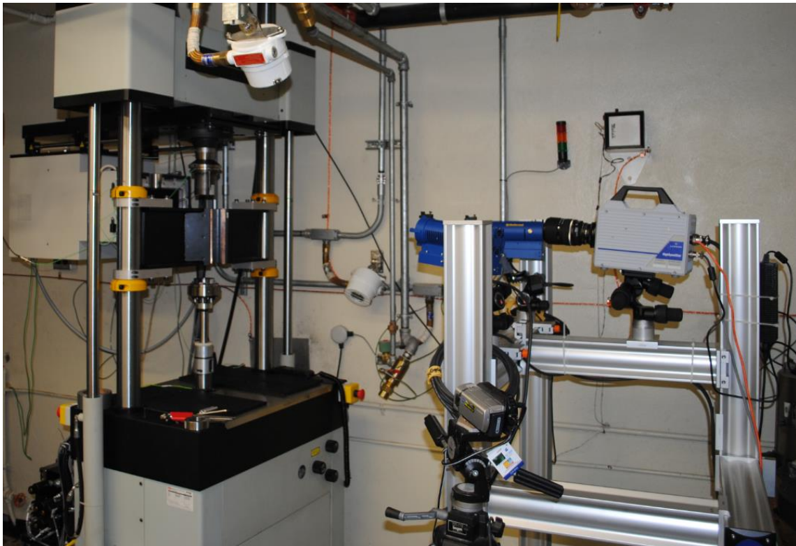
Figure 1 High-rate material testing device with high-speed camera measuring actuator displacement
