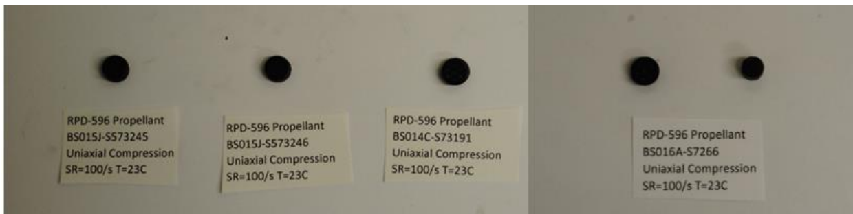
Figure 4 RPD-596 samples post-test at 23°C and an undeformed grain on the right
