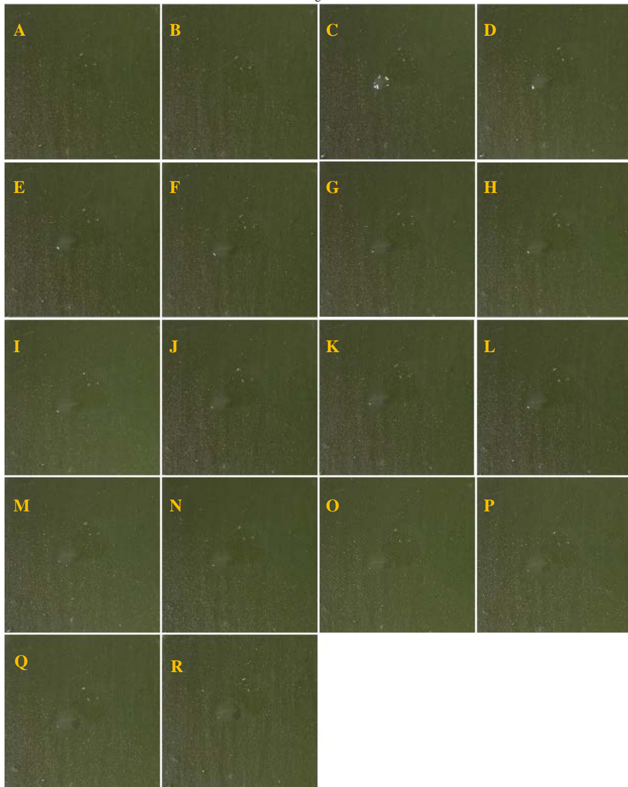
Fig. B2 — MES on Fomblin Y oiled paint. Images of a coupon before application (A) and at 0 (B), 0.5 (C), 1 (D), 1.5 (E), 2 (F), 2.5 (G), 3 (H), 3.5 (I), 4 (J), 4.5 (K), 5 (L), 5.5 (M), 10 (N), 15 (O), 20 (P), 25 (Q), and 30 (R) min following application of the target.
