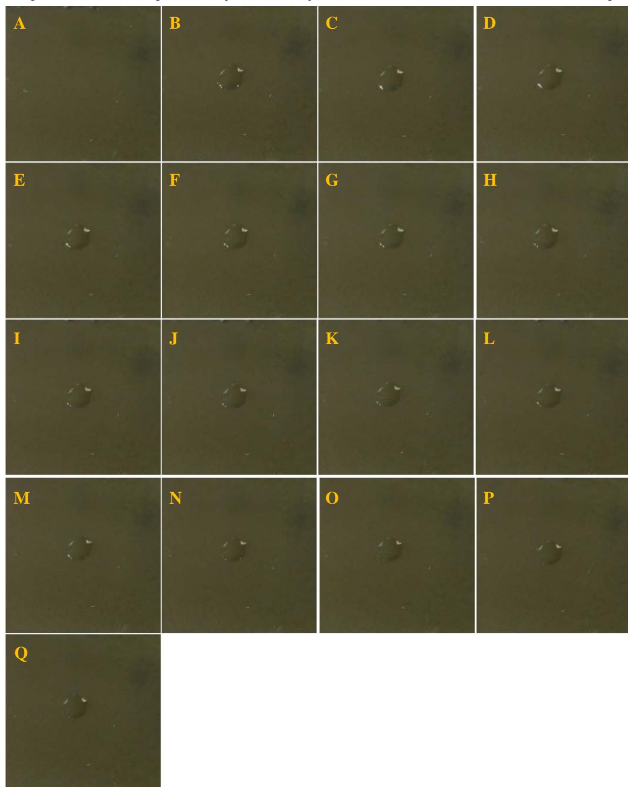
Fig. D1 — DFP on Gentoo coating. Images of a coupon before application (A) and at 0 (B), 0.5 (C), 1 (D), 1.5 (E), 2 (F), 2.5 (G), 3 (H), 3.5 (I), 4 (J), 4.5 (K), 5 (L), 10 (M), 15 (N), 20 (O), 25 (P), and 30 (Q) min following application of the target. These images were collected with a glass cover in place to limit evaporation. Reflections from the cover can be seen in some images.
