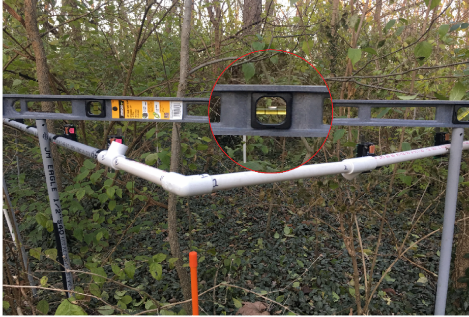
Figure 3.2. Image showing the stakes being level and parking marker at location [0,0]
