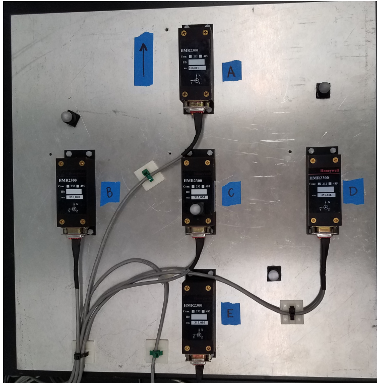
Figure 9. AFIT Tensor Measurement Assembly
