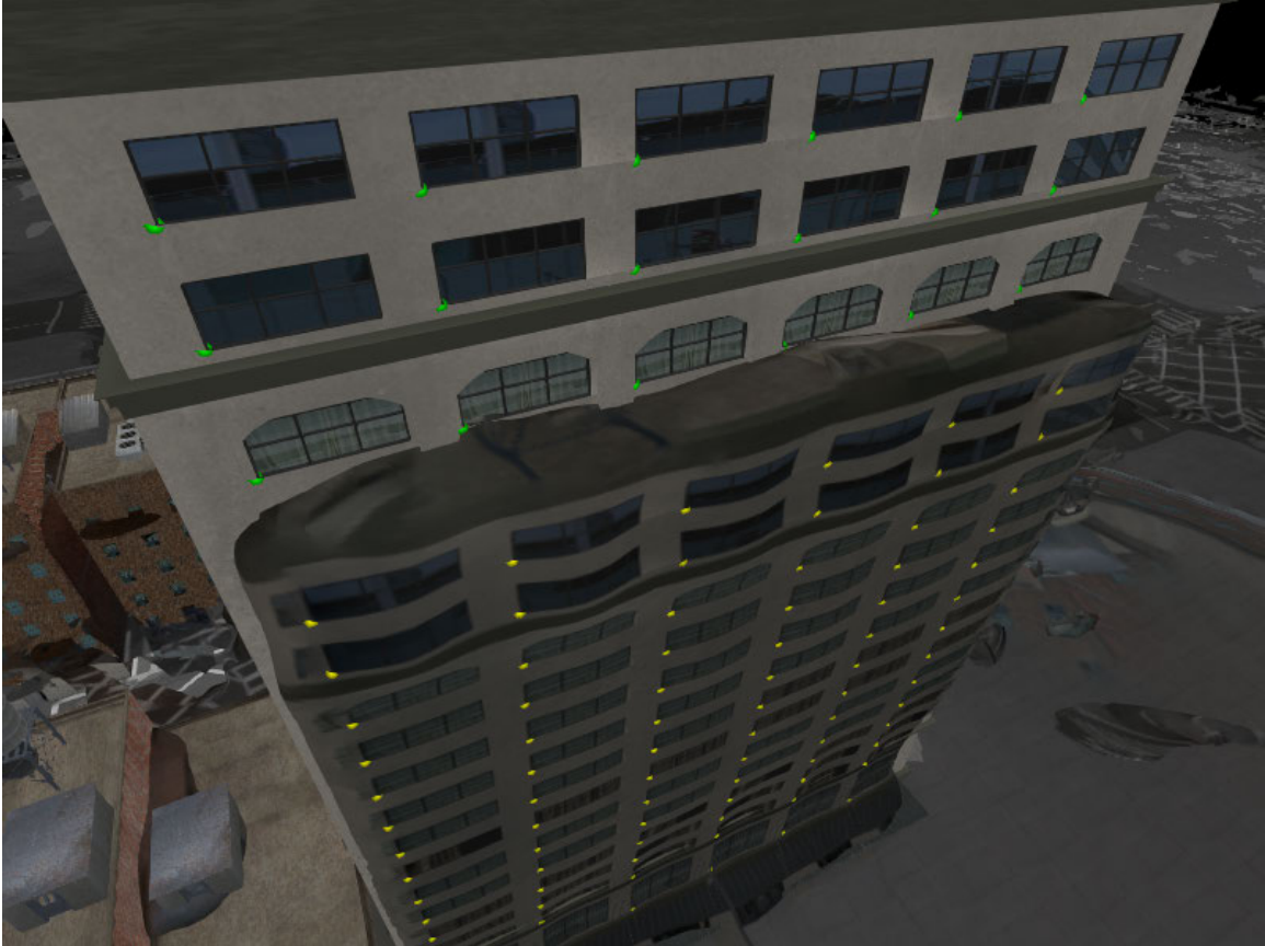
Figure 19. Visualization of geoints; green dots represent truth data, and yellow dots represent reconstruction data. The spatial difference between each corresponding pair quantifies the distortion of the reconstruction.
