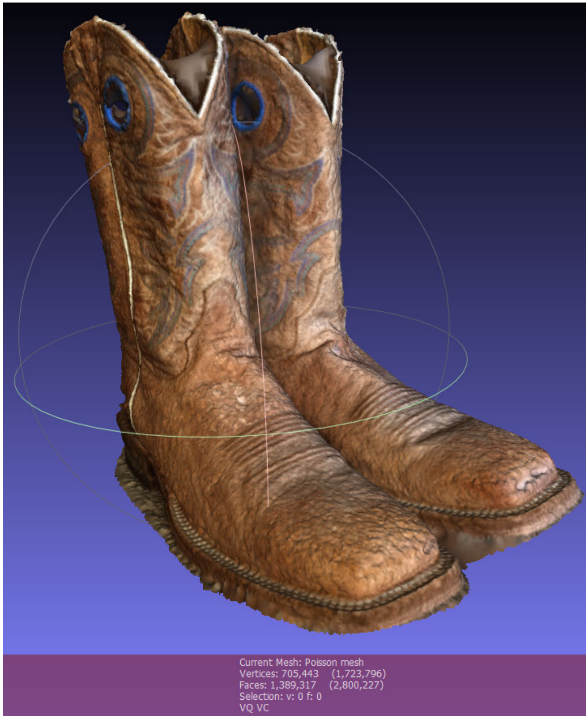
Figure 8. A Poisson Reconstruction of the model, performed in Meshlab
