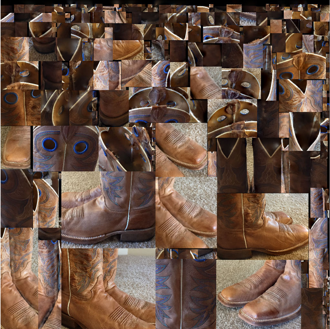
Figure 11. The source image for texturing the model; automatically generated in Meshlab from pieces of the input images
