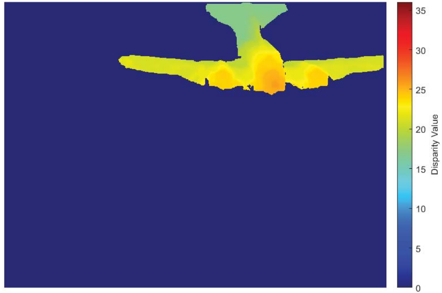
Figure 24. Disparity Map Generated from the Images in Figure 23.
