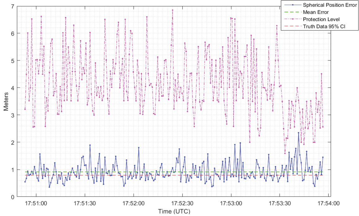
Figure 133. V5 Spherical Position Error on Flight Test Data Using a Uniform Prior.
