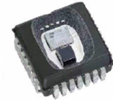
Figure 1: BOSCH high-g accelerometer for vehicle airbag system from 1990s [5].
