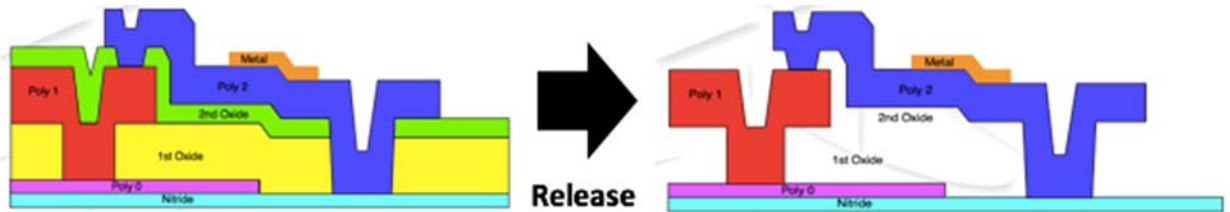
Figure 18: Diagram showing how sacrificial PSG layers are removed during release etch [18].
