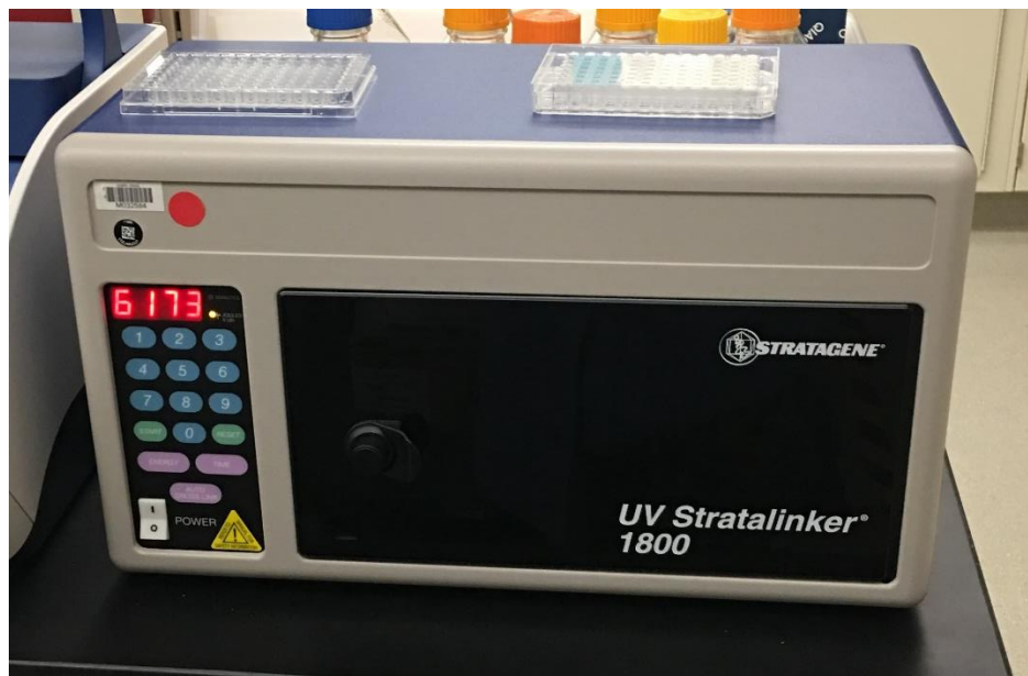
Figure 7. Stratalinker 1800 used to impart 9999 \text{ J m}^{-2} of UV energy onto the samples.
