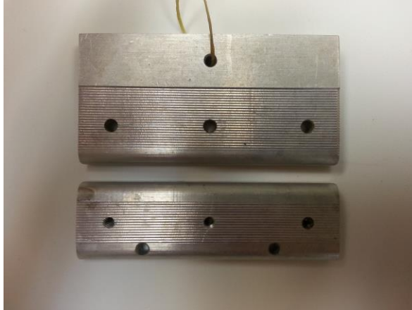
Figure 10. Textured aluminum clamping device to grip Achilles tendon.
