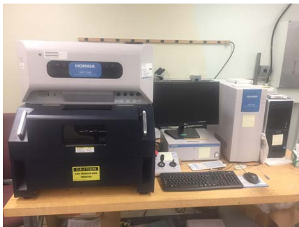
Figure 12. Horiba Scientific XGT-7200 XRF imaging microscope.
