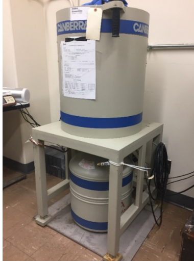
Figure 16. HPGe Detector assembly mounted over liquid nitrogen dewer.
