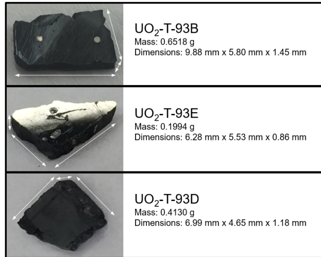
Figure 9. Dimensions of samples \text{UO}_2 -T-93B, -93D, and -93E.
