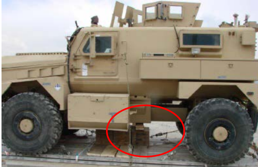
Figure 6: Shoring for Rolling Stock
