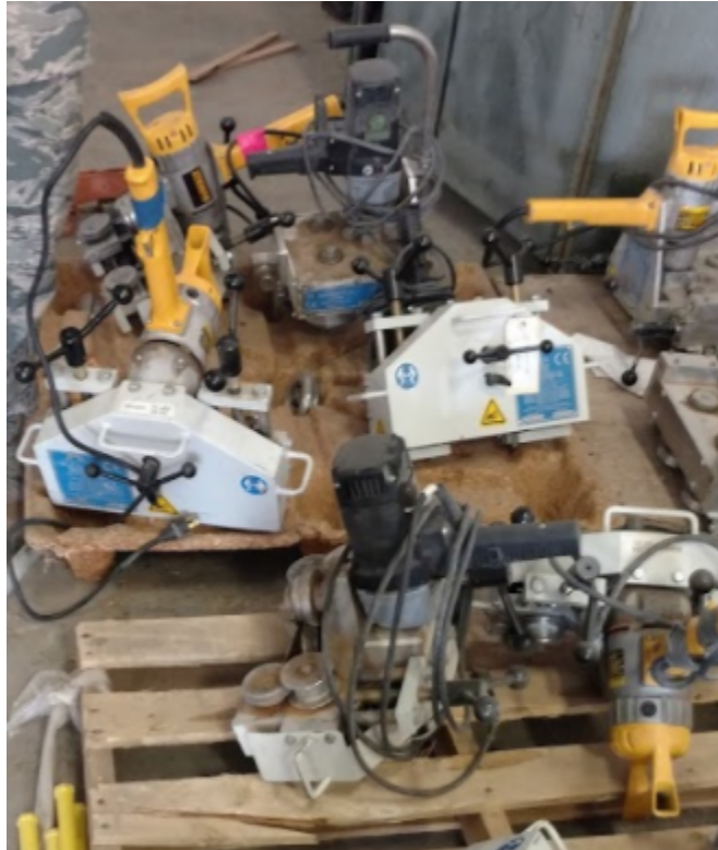
Figure 2.10: K-Span Panel Seamers - Nellis AFB, NV
