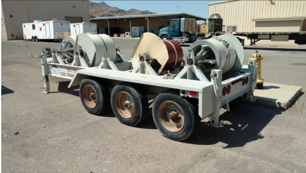
Figure 2.9: Coil Transport Unit - Nellis AFB, NV
