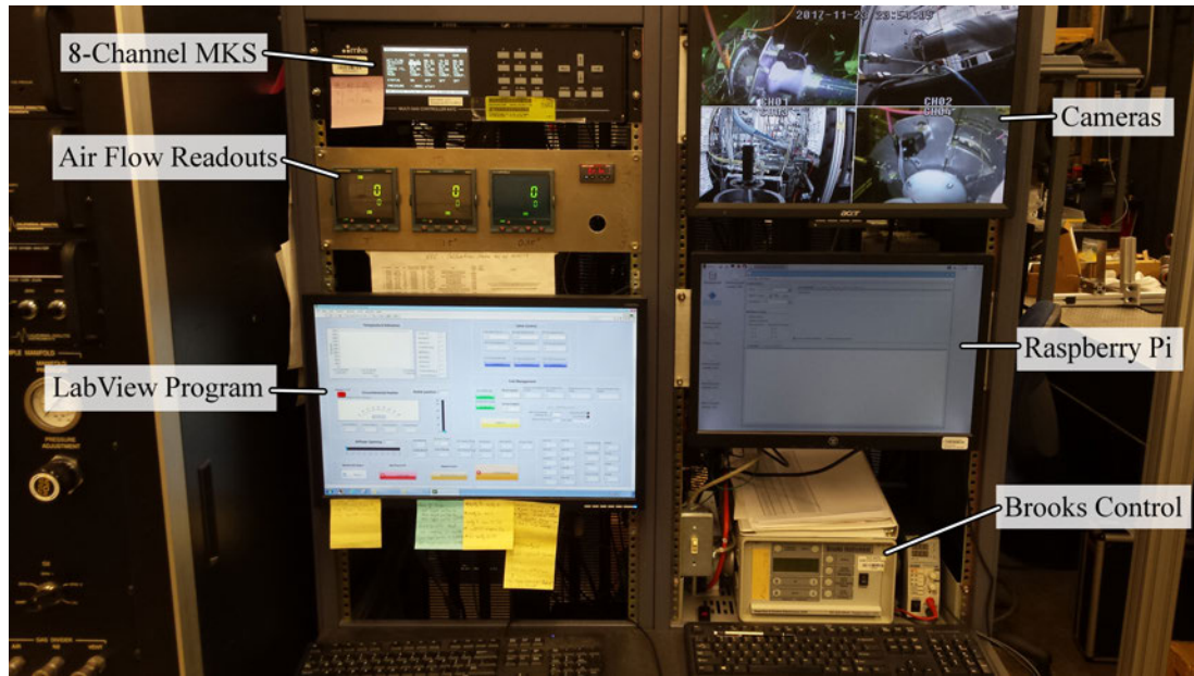
Figure 29. UCC Control Station
