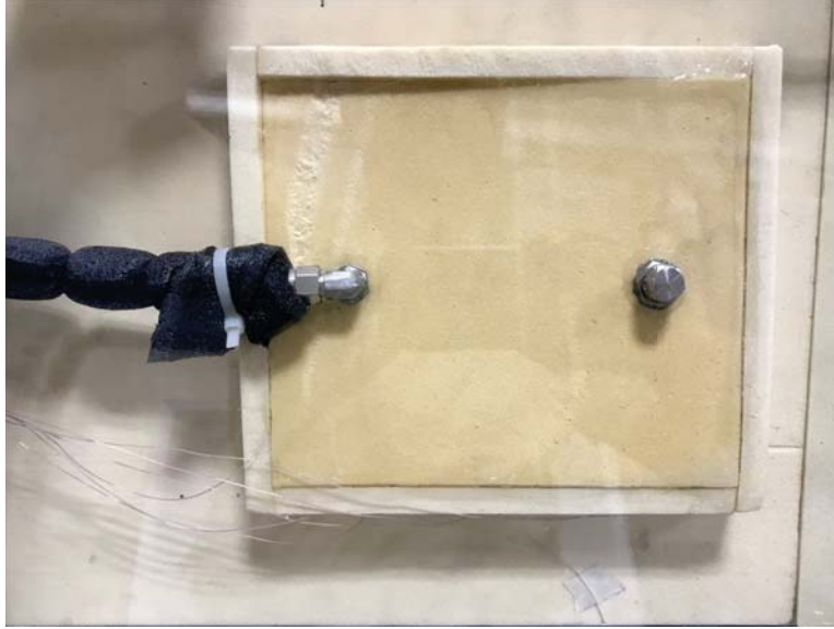
Figure 3.6. First plenum constructed for the single hole test insert, mounted behind test surface.
