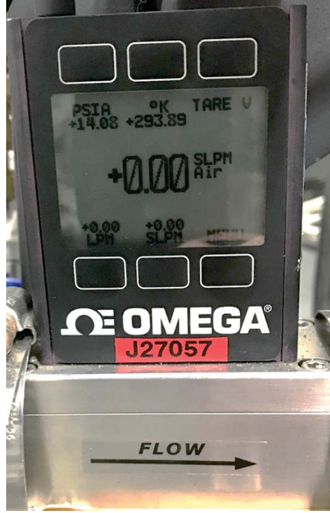
Figure 3.11. Omega flowmeter used to monitor flow rates.
