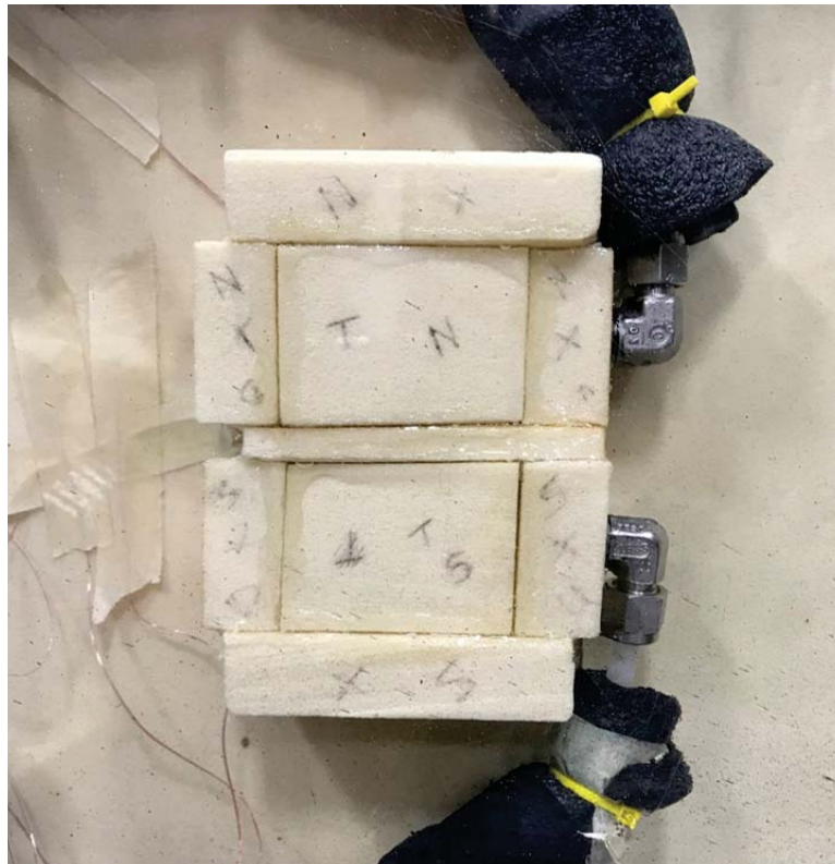
Figure 3.10. Plenums constructed for the two hole test insert.
