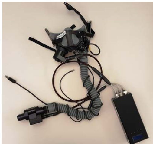
Figure 11: AMPSS 2.5 - Modification to MBU-20/P Flight Mask
