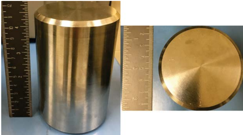
Figure 3.13. An upsetting workpiece preform machined to 3in diameter x 4.5in length
