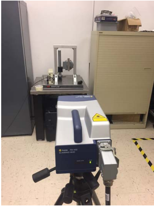
(a) Laser Vibrometer Test Setup
