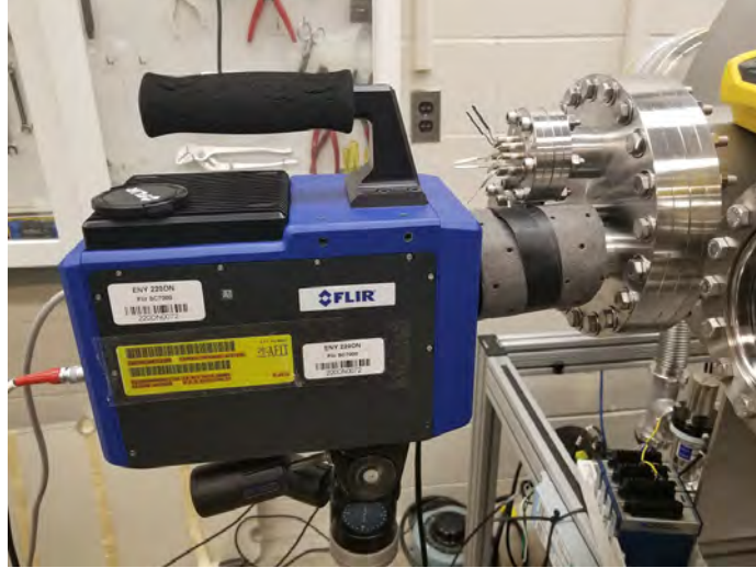
Figure 3.35: FLIR SC7000 IR camera and MWIR L0106 lens used for testing mounted to Germanium viewport window on vacuum chamber
