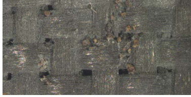
Figure 35. Voids in the matrix located at fiber cross-overs on the surface of the composite specimen 5-7-C-2-3 with Type 2 geopolymer matrix.
