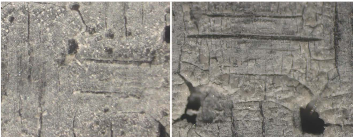
Figure 27. Microcracking of matrix on surface of 5-7-C-14 Type 2 geopolymer matrix specimen before thermal exposure (left) and after (right).
