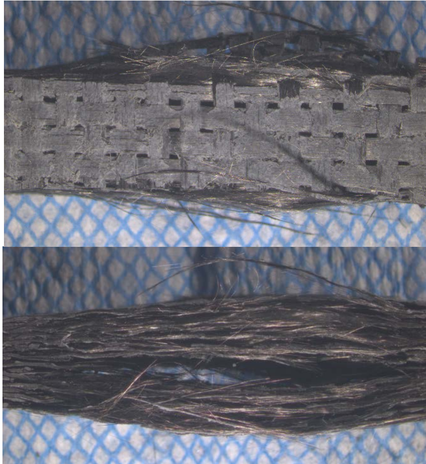
Figure 22. Specimen 5-7-C-1-3, failed in tension test at 23°C.
