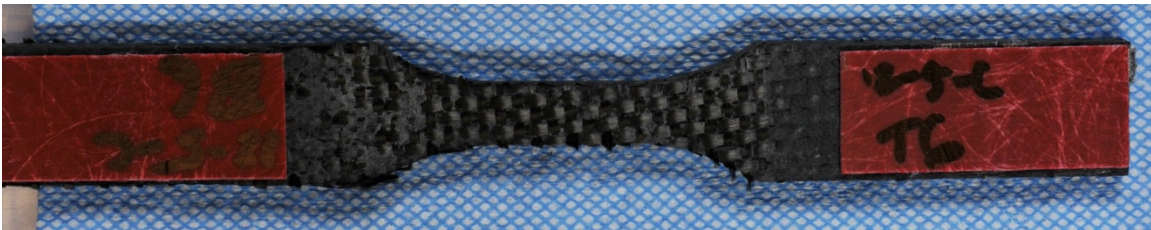
Figure 9. Test specimen with fiberglass tabs, from panel 12-5-C.
