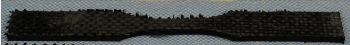
Figure 8. As-machined specimen from panel 3-20-C.
