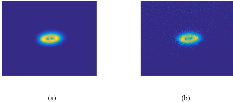
Figure 4.7. (a) Experimental data image processed from the mean of 100 noisy PSF images. (b) One of the 100 noisy frames used to create the target PSF.
