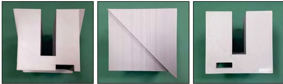
Figure 20. New cavity rear design. Small channel at the floor of the cavity prevents bunching of the wiring by allowing the linear motor's wiring to lie flush with the deck. The left picture is a view from the inside of the cavity looking aft the center picture is a side profile view and the right picture is from behind the cavity looking forward.
