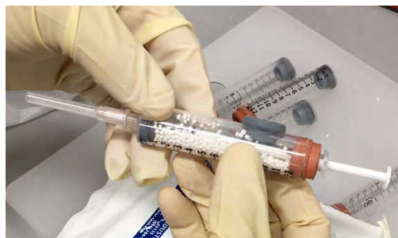
Figure 7. Photograph of loaded prototype Gen 1.0 hydrogel tool prepared for the workshop. Improvements suggested by the workshop participants included finger loops for improved control and manipulation, Luer lock tip for tip placement, and window for seeing hydrogel quantities released.
