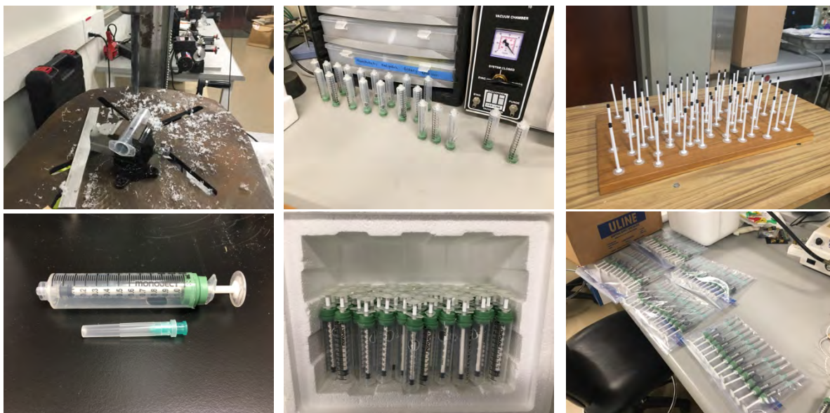
Figure 8. Selected photographs showing the production steps for manufacturing the prototype injector tools for the Walter Reed workshop. Circular holes were machined into 12cc syringes to create the outer thermal jackets. Green stopper plugs were machined to create the upper flange through which the 1cc syringes were inserted. 1cc syringe plungers were modified by adding a larger thumb plate for better pressure application during injection. The completed tools were collected, quality checked and packaged in groups of one dozen, for shipment.
