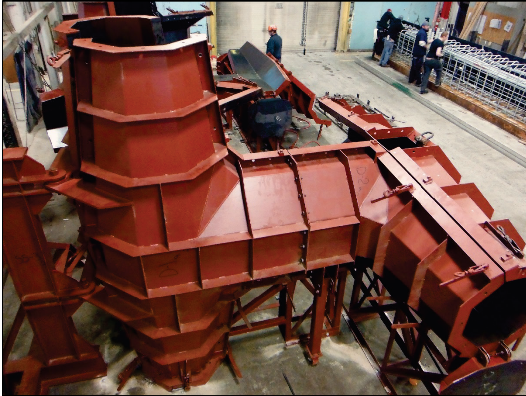
Figure 3-4. Oswego Detached Breakwater 16-ton dolos form.
