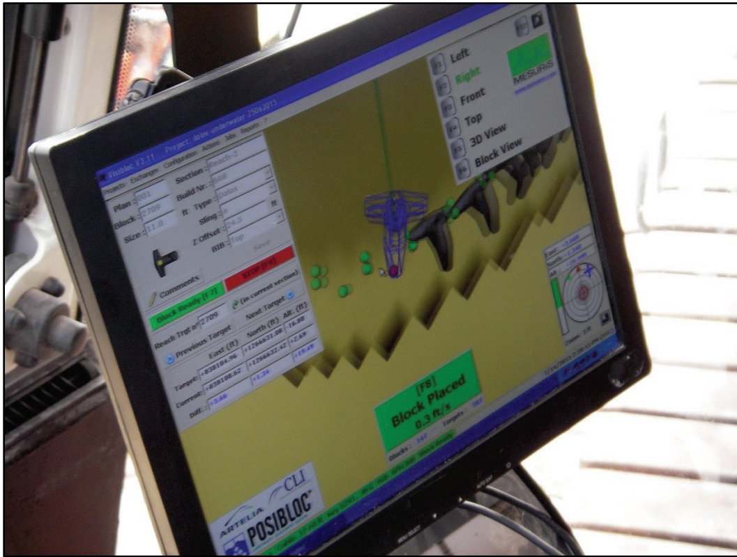
Figure 4-3. Crane operator’s view of computer screen during Oswego dolos placement.
