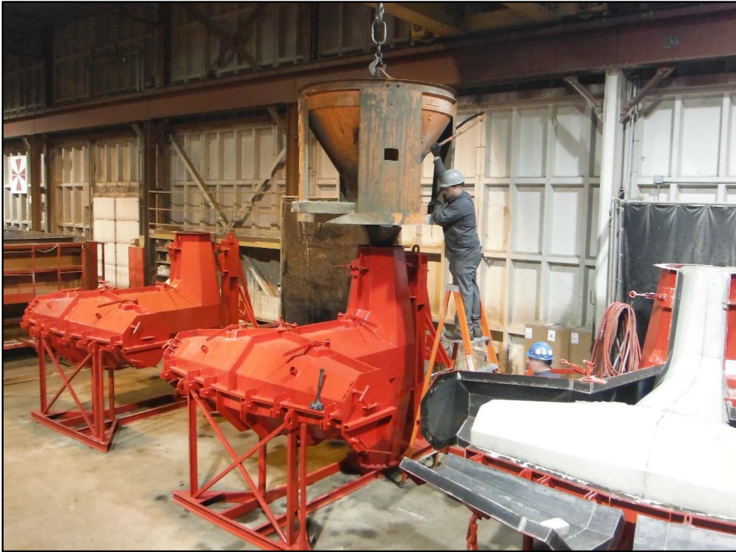
Figure 3-6. Placing concrete for Cleveland 6.5-ton dolos.
