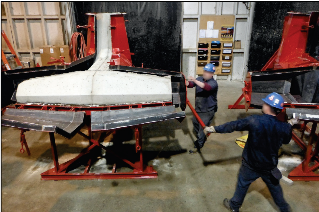
Figure 3-9. Opening Cleveland 6.5-ton dolos form side wings.
