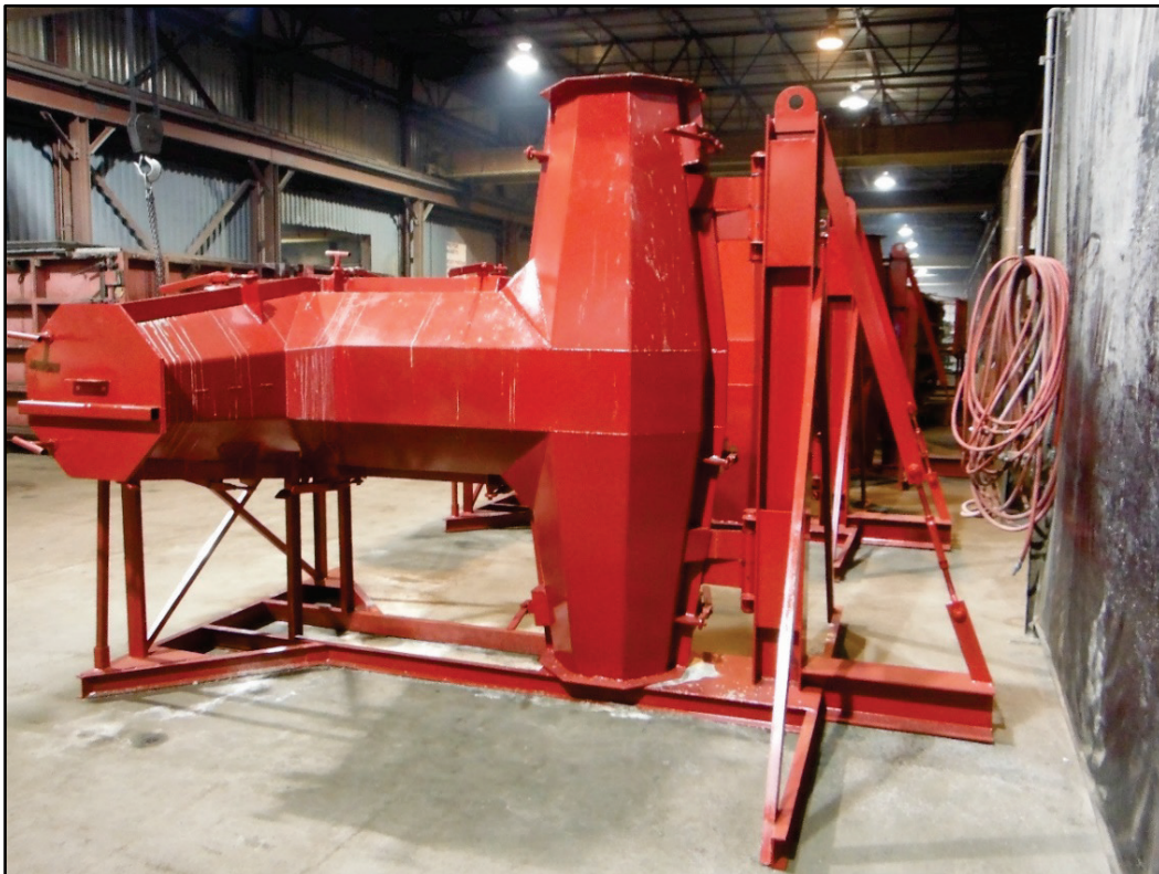
Figure 3-3. Completed Cleveland 6.5-ton dolos forms.
