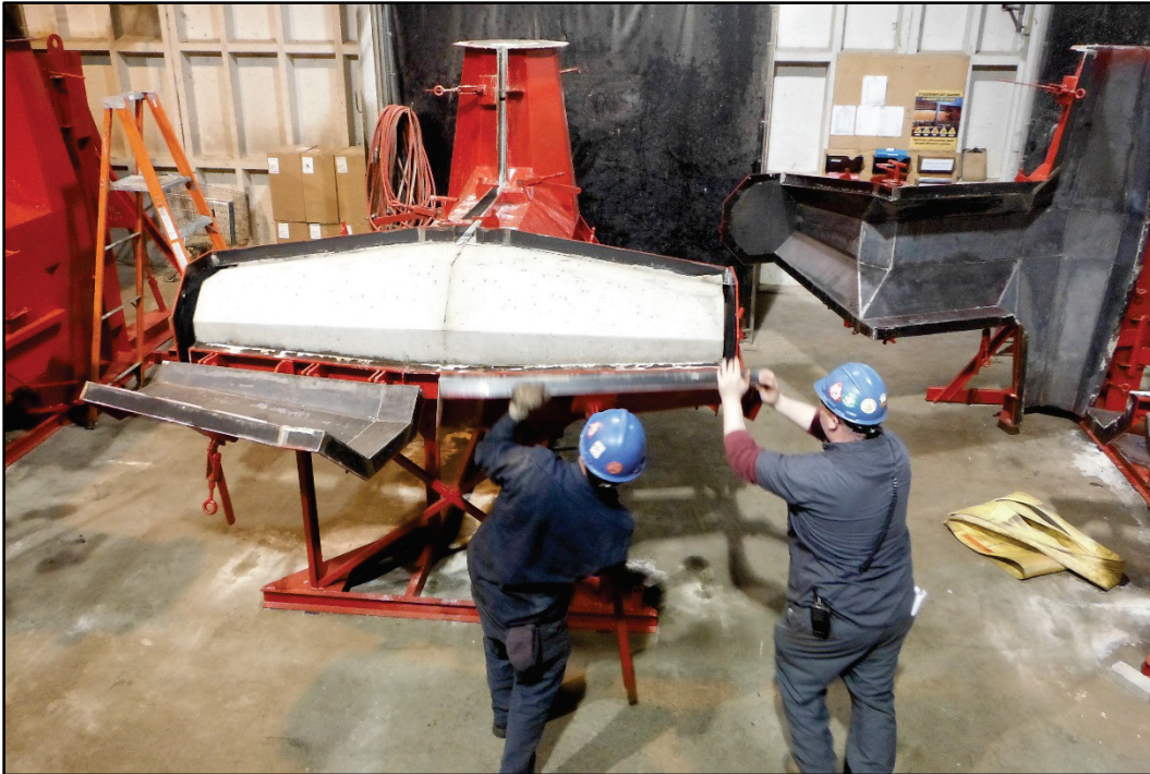
Figure 3-8. Opening Cleveland 6.5-ton dolos form fluke flaps.
