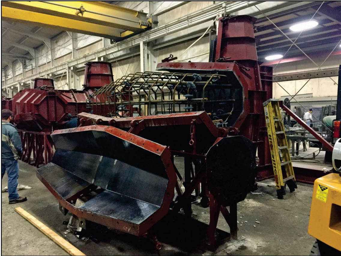
Figure 3-5. Oswego Detached Breakwater 16-ton dolos form.
