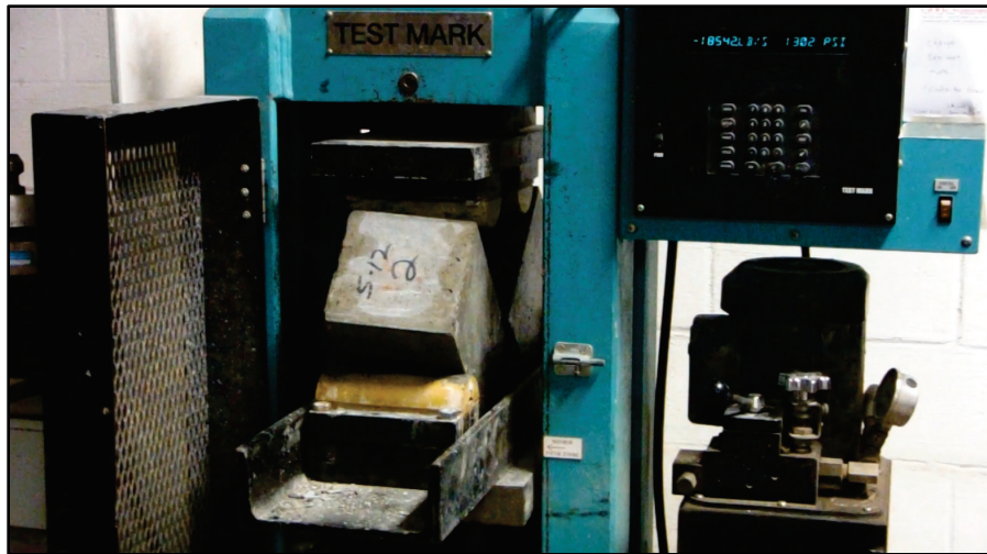
Figure 3-21. Cleveland dolos 28-day flexural strength test (sample failed at 1,302 lb/in. 2 ).
