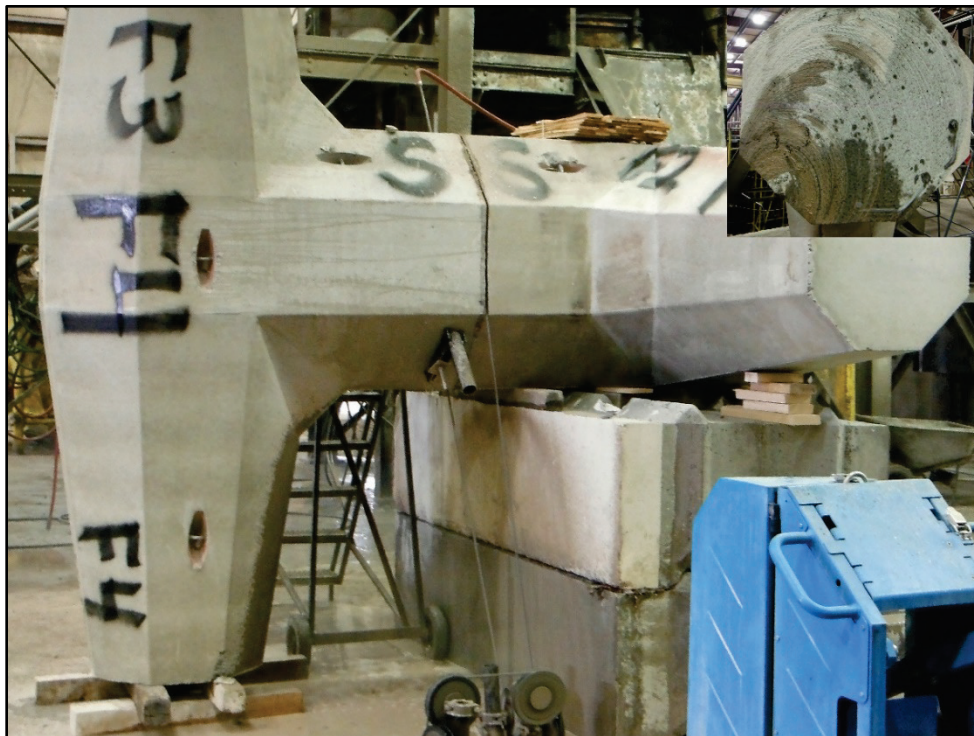
Figure 3-14. Cutting Oswego 16-ton dolos and cut sample.
