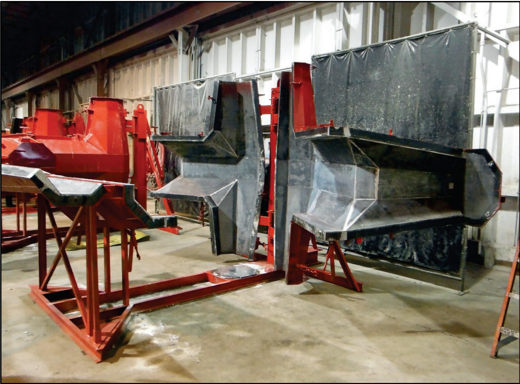
Figure 3-11. Cleveland 6.5-ton dolos empty open form.
