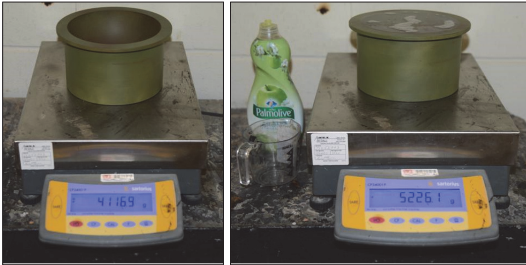
Figure 19. Water calibration of aluminum bowl insert, empty (left) and filled with water (right). Soap was added to create a level surface.
