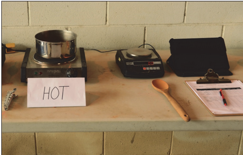
Figure 25. Hot plate, scale, and accessories used to determine soil moisture content.
