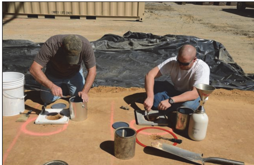
Figure 30. Testing of sand cone density and photogrammetry technique inside red ring. Sharpshooter shovel was used for some photogrammetry excavations.
