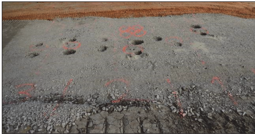
Figure 32. 12 post-test locations of sand cone and photogrammetry samples on Limestone test section for both low and high compaction efforts.
