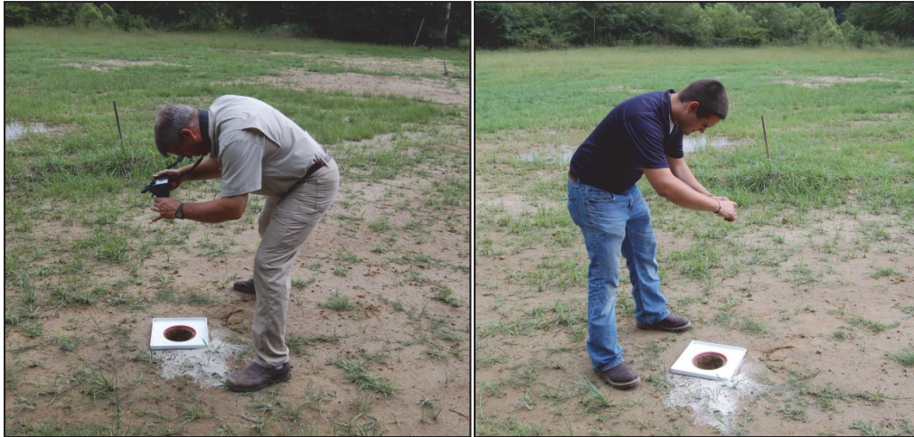
Figure 5. Example of photographing hole to obtain imagery for processing. Note a red ring was painted onto a sand cone plate for scaling and for comparative density purposes. A digital SLR and a point-and-shoot digital camera were both used for comparative purposes of pixel density.
