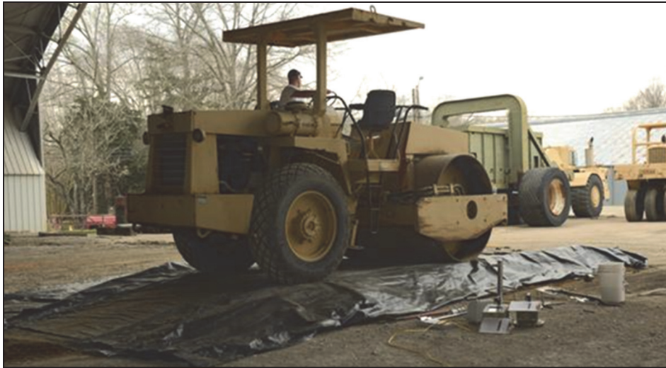
Figure 28. Use of plastic sheet on test strip to prevent soil adhering to the drum.
