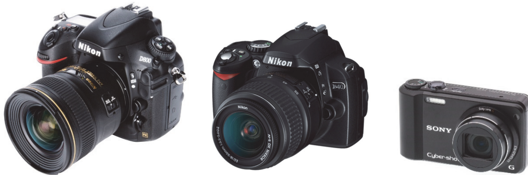
Figure 21. Cameras used in calibration experiment: Nikon D-800 (left), Nikon D-40 (center), Sony DSC-H70 (right).
