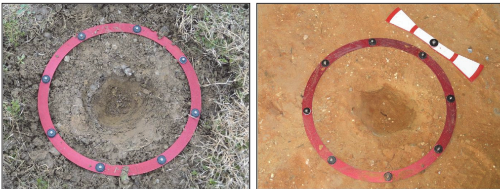
Figure 4. Plan views of excavated holes and typical scales used for obtaining distance in the photographs (circular red ring or horizontal bar shown). Note the color red is used to provide good contrast with the surrounding soil.
