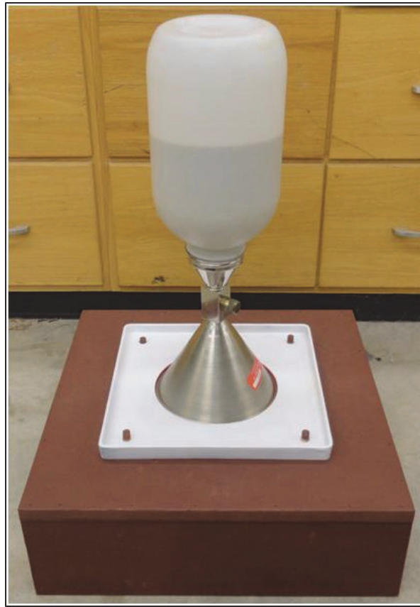
Figure 20. Sand cone mounted on the calibration platform.
