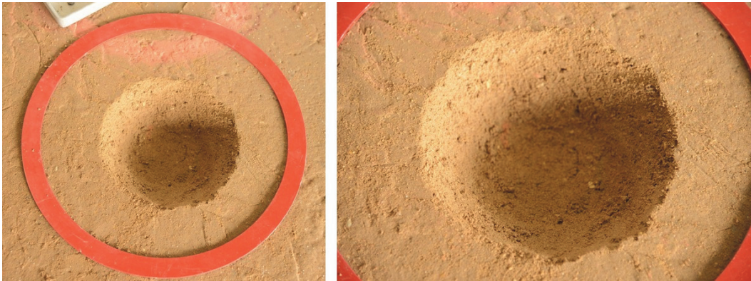
Figure 38. SC-Blended clayey sand soil excavation.
