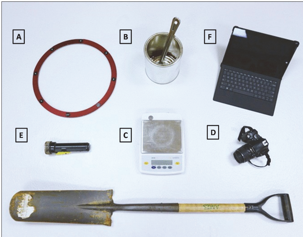
Figure 1. Components required to perform a photogrammetric analysis of soil density.
