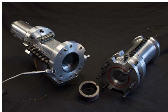
Figure 18 – Photographs of the axisymmetric scramjet combustor model
