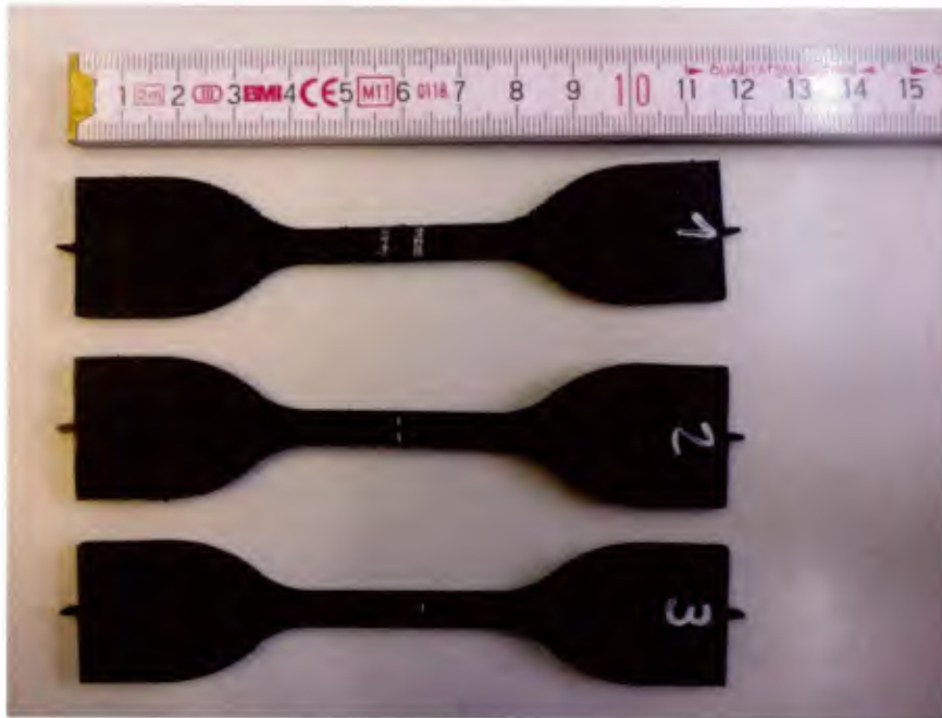
Figure 91: Dumbbell-shaped rubber specimens
