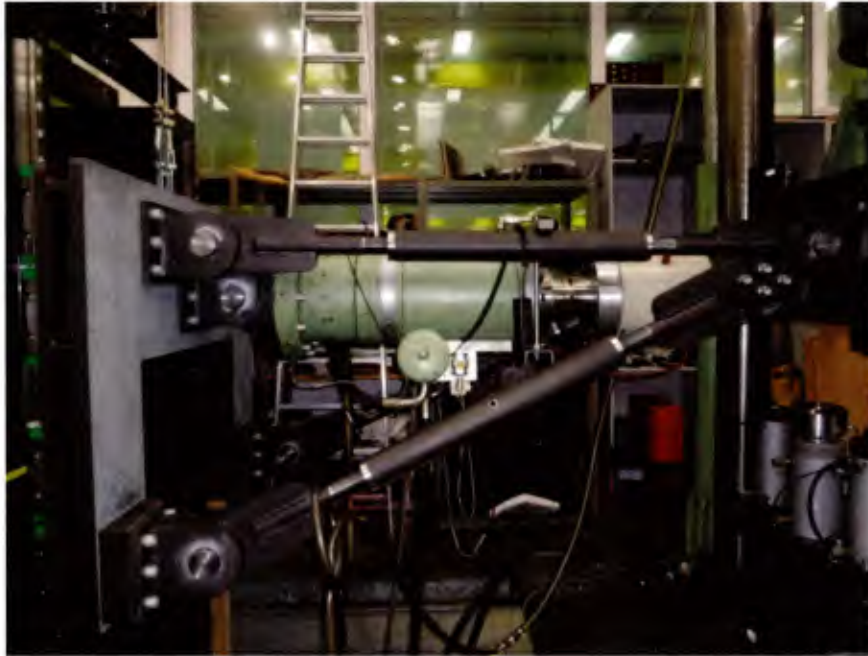
Figure 55: Support construction for the left (upper) horizontal actuator
