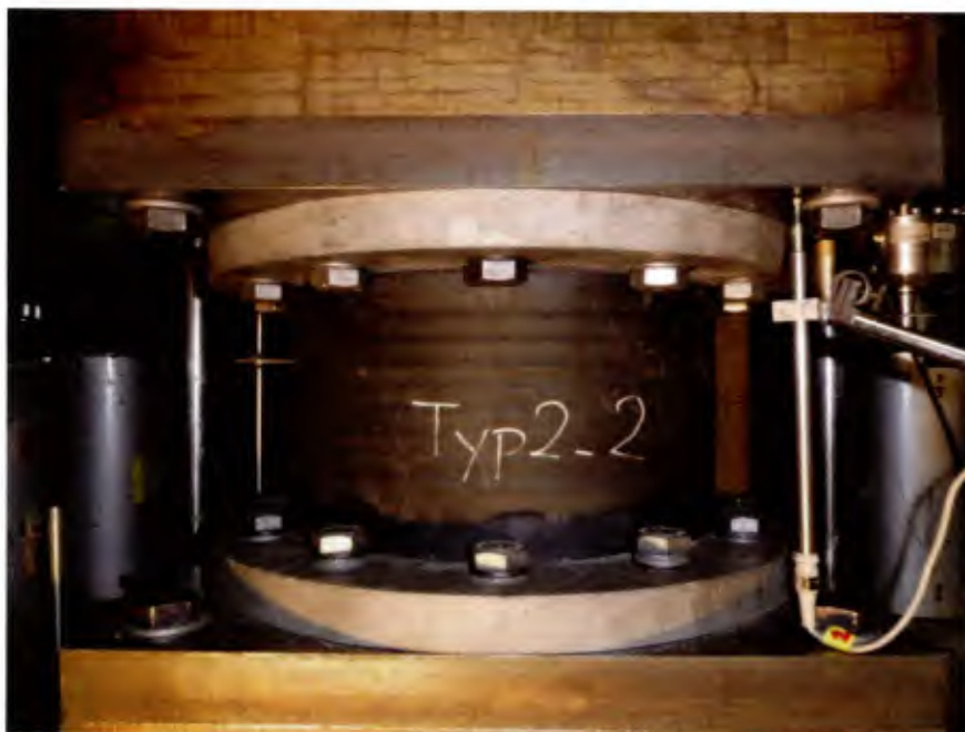
Figure 69: The bearing 2-02 during the uniaxial tension test
