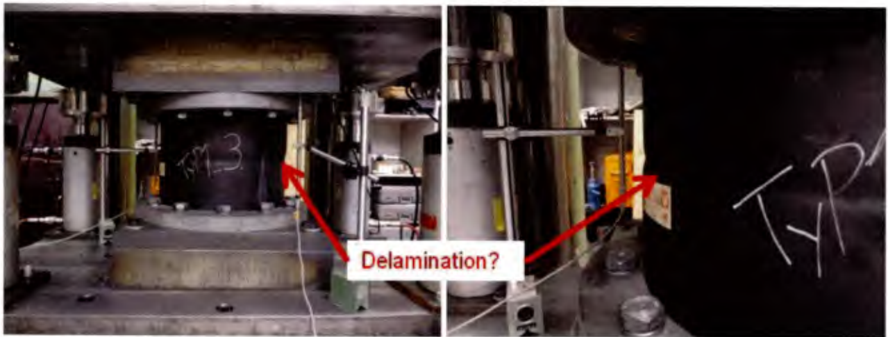
Figure 68: Visible damage of the bearing 1-03 during the uniaxial tension test
