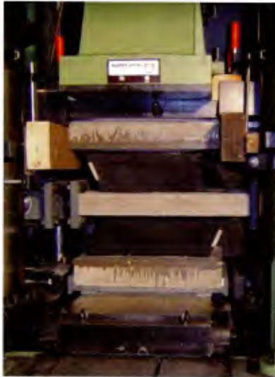
Figure 30: Tested laminated elastomeric bearing and their hysteresis curve [4]
