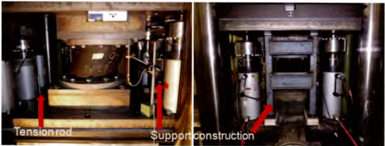
Figure 57: Test setup for the offset tension test
