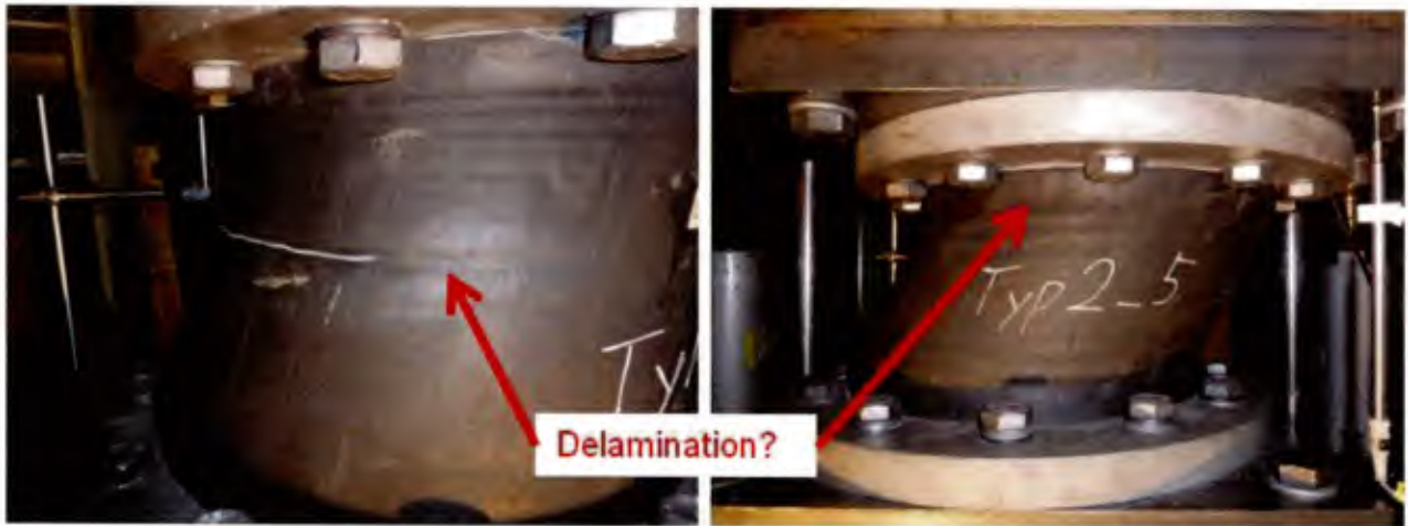
Figure 72: Visible damage of the bearing 1-09 (left) and 2-05 (right) during the offset tension test
