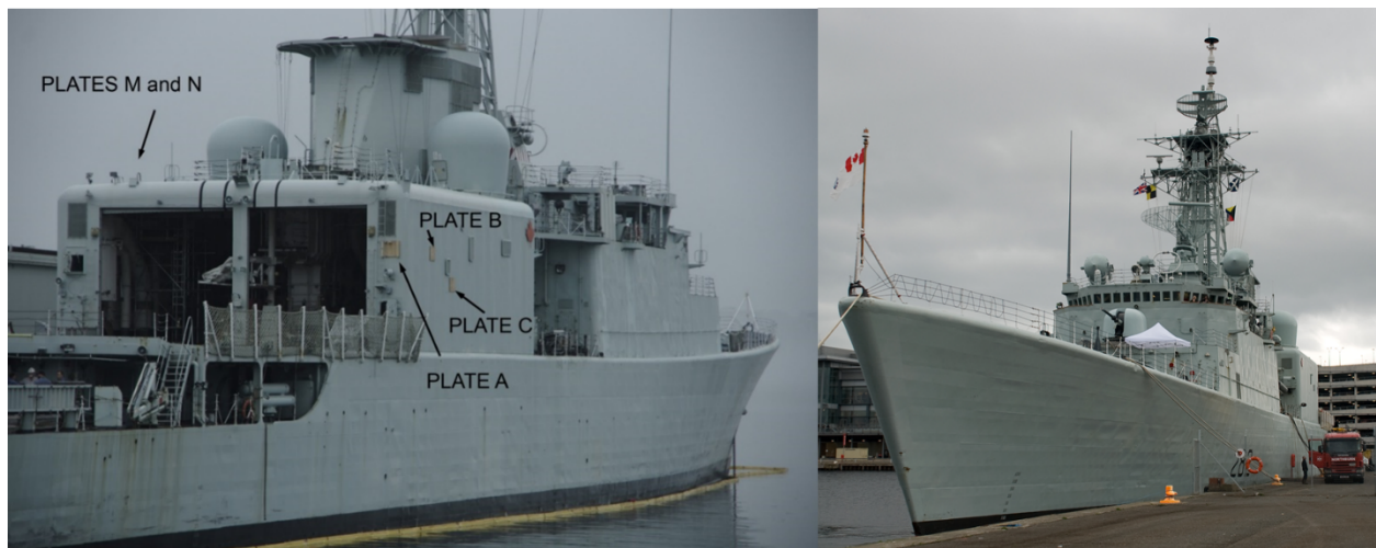
Figure 7: Two Iroquois class destroyers. The HMCS Iroquois (left) with 42 years of service, showing regions from which plates have already been removed and initial testing at CWRU has begun. Material from the HMCS Athabaskan (right) with 45 years of service may become available at some point.
