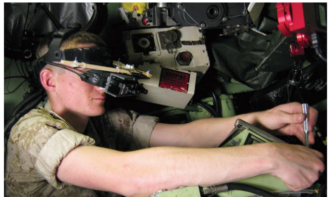
Figure 3 While wearing a tracked, head-worn display, a mechanic to complete a maintenance task inside an LAV-25A1 armored personnel carrier.
