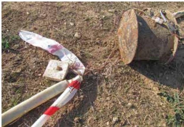
The same PPIED after neutralization. Note the square, white electronic anti-lift device on the left.
