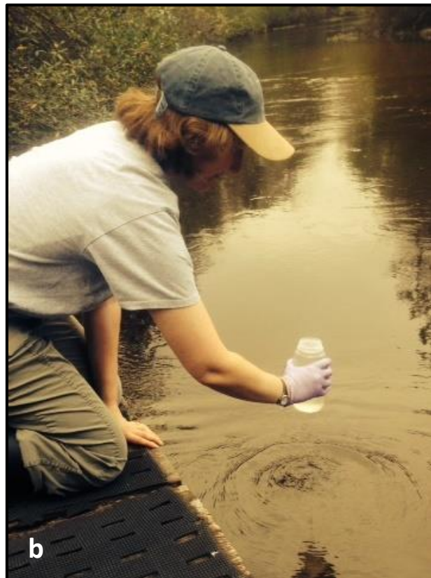
Figure 8. Collect water in (a) disposable Whirl-Pak® bag or (b) decontaminated Nalgene bottle.
