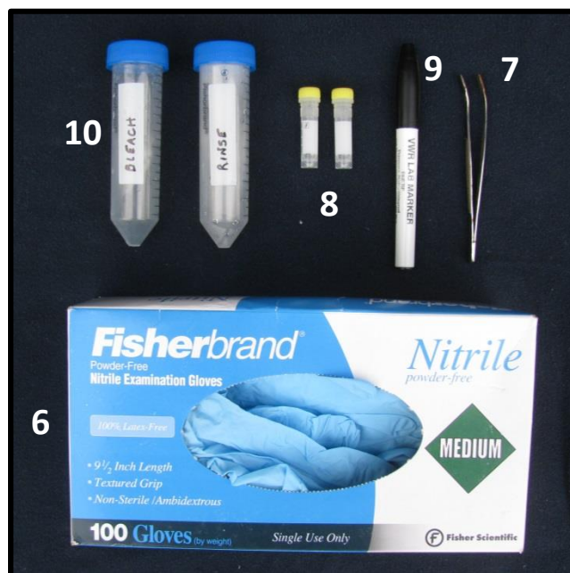
Figure 2. Latex or nitrile gloves (6), forceps (7), 2 mL o-ring tubes with 1 mL ethanol (8), ethanol-proof lab marker (9), and 2 50 mL tubes with 50% household bleach/distilled water solution (10).
