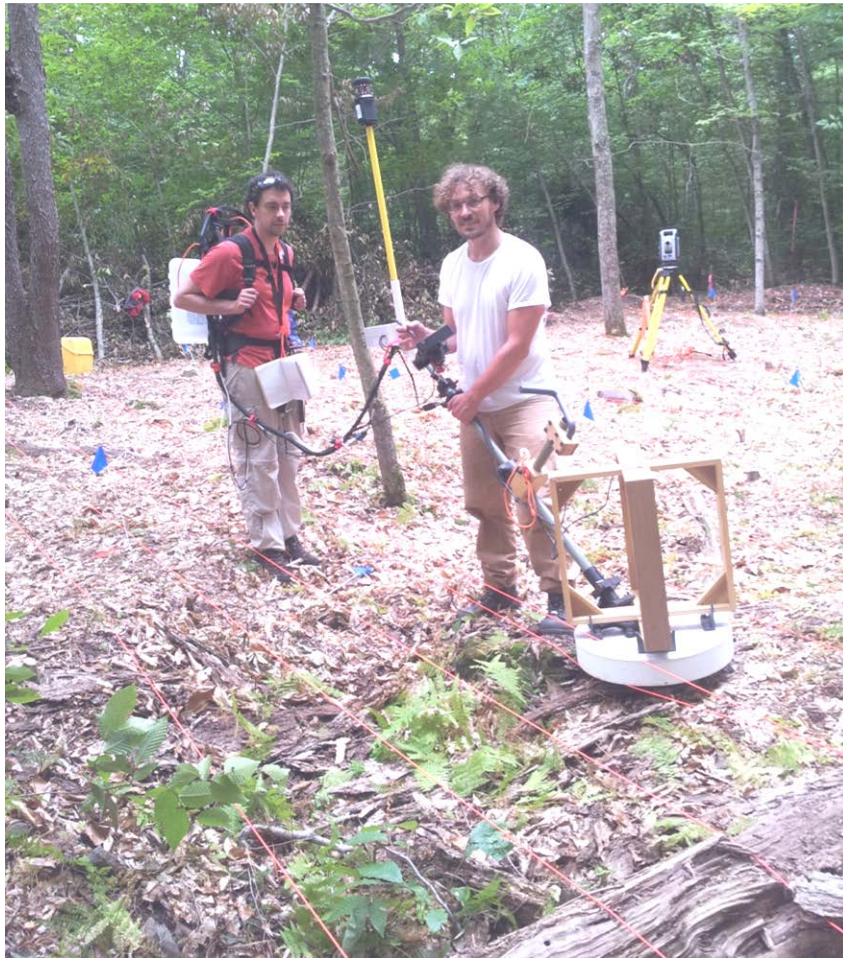
Figure 3. MPV in Cued Interrogation Mode with Detachable Coils for 3D Excitation of Buried Targets.
