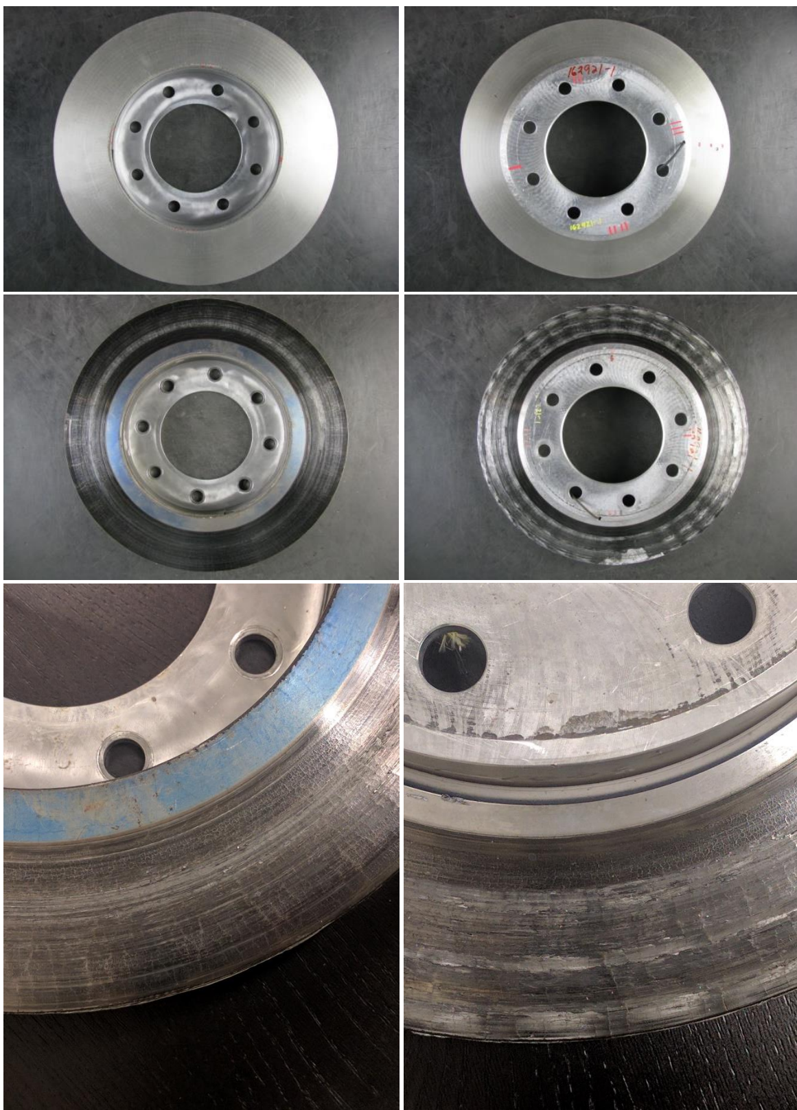
Figure 3. Coated aluminum rotor- Inboard side (L) and Outboard side(R)
