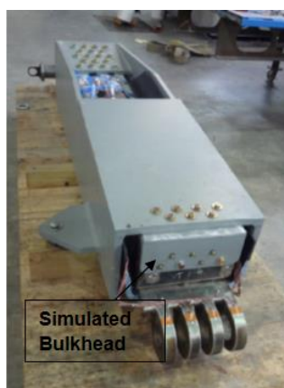
Figure 3. Joint Test Specimen within Steel Box
