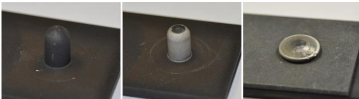
Figure 34. Photos of MGC-2.0 treated Mg lap-shear tension coupons (a) prior to contact by the electrode, (b) after application of initial contact force by the electrode but prior to application of electrical current, and (c) after full forming operation with force and current
