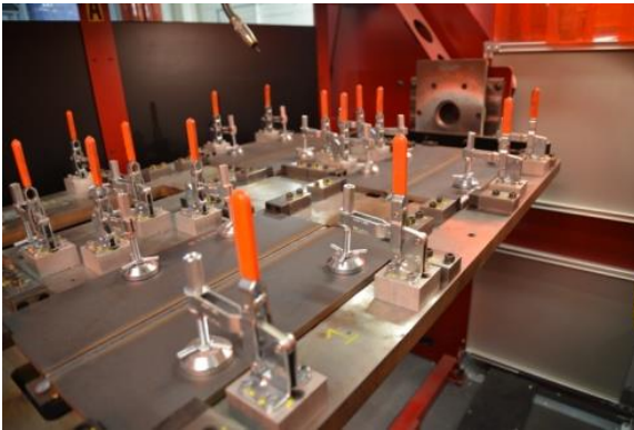
Figure 1. Fixture for Robotic Welding of Phase I Plate
