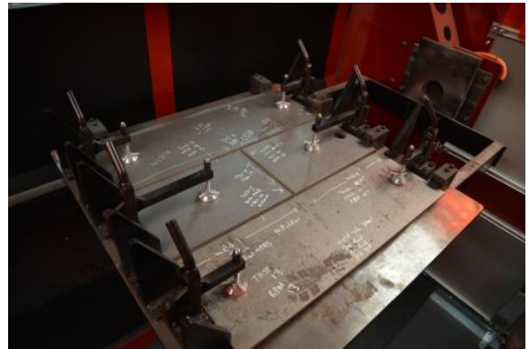
Figure 2: Phase II H-Plate Clamped and Ready for Welding
