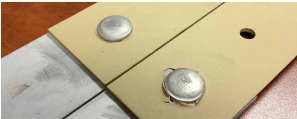
Figure 33. Photo of two joined lap-shear tension assemblies utilizing the CARC coating on the steel coupons
