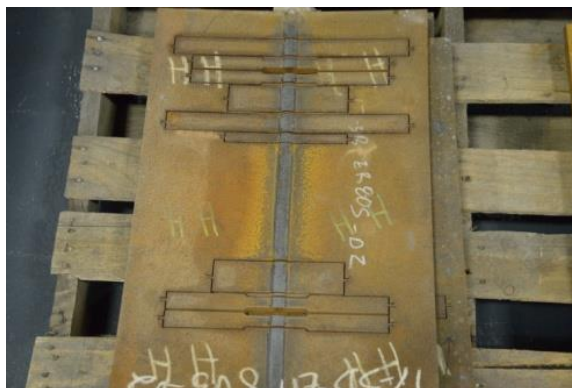
Figure 6. Phase I-Plate Marked Samples for Standardized Weld Characterization Tests
