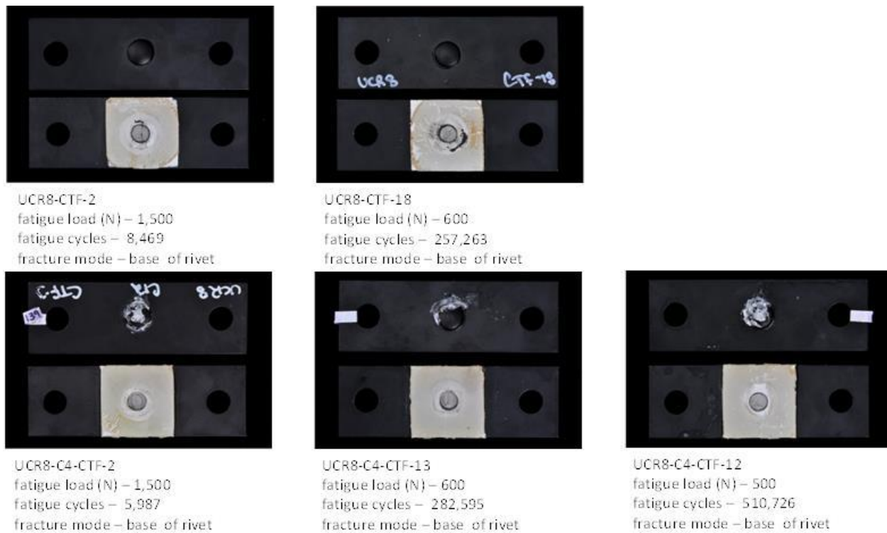
Figure 32. UCR fatigue cross tension (CT) test assembly failure mode prior to corrosion exposure (top) and after 4-weeks of accelerated corrosion exposure (bottom). Typical failure is at base of rivet.
