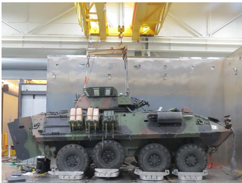
Figure 2. Lift Fixture Attached to the Multi-Material Turret.
