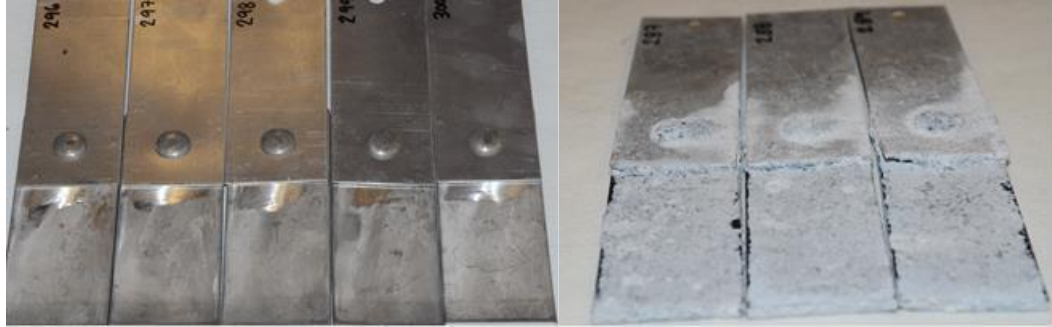
Figure 8. UPJ7-1 bare Mg to bare Al lap shear tension test coupons before corrosion exposure (left) and after 12-weeks of exposure (right)
