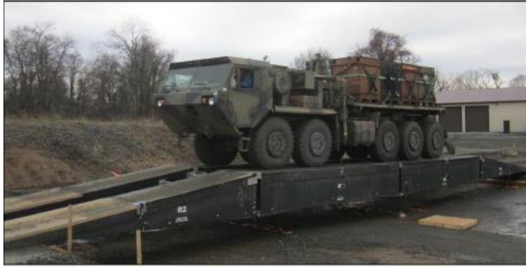
Figure 5. Fully Loaded PLS crossing over the AMCB
