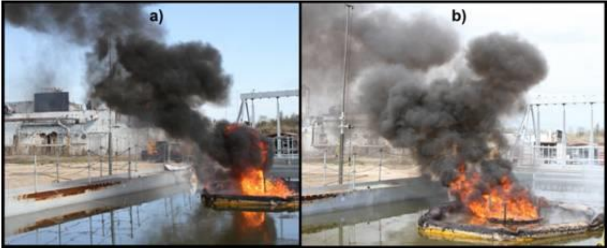
Figure 8. Picture of the smoke plume a) baseline, b) blanket with 48 coils (VH).
