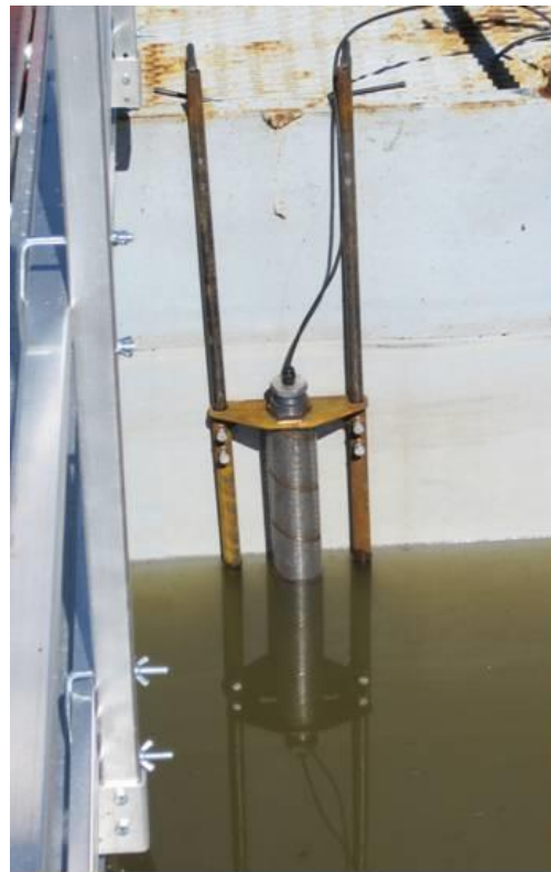
Figure 10. Wave height measurement device.
