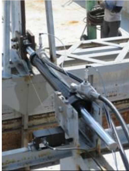
Figure 11. Close up of hydraulic cylinder.
