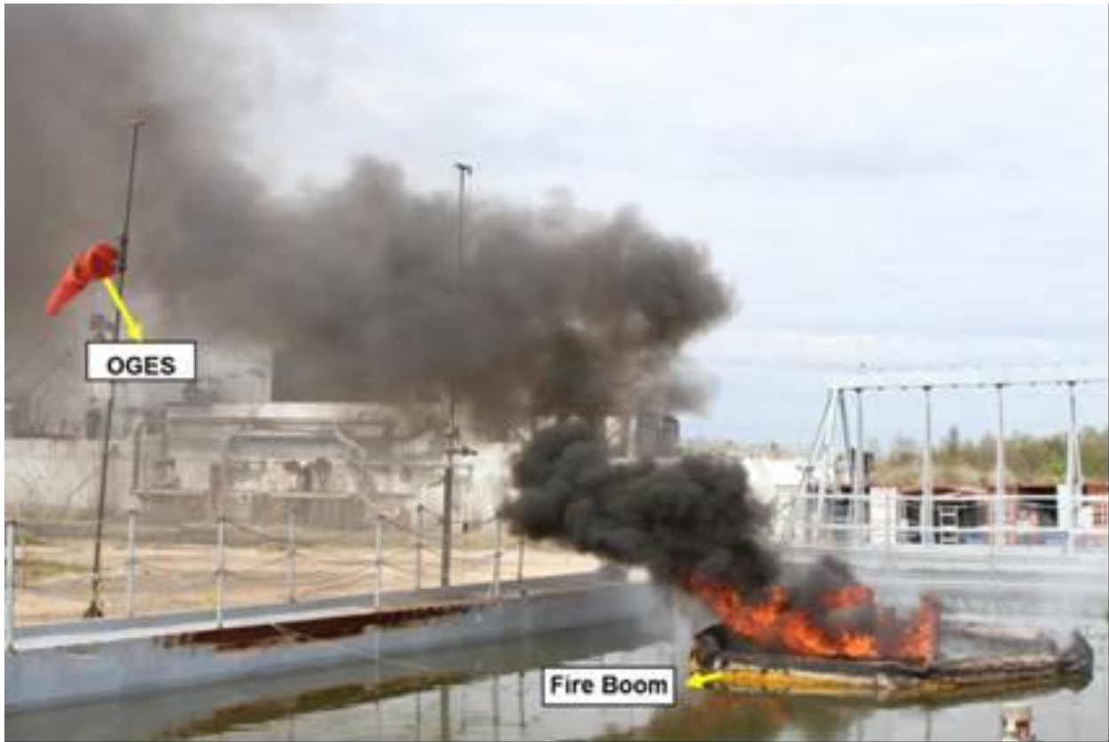
Figure 7. Outdoor Gas Emission Sampling System (OGES) in place.
