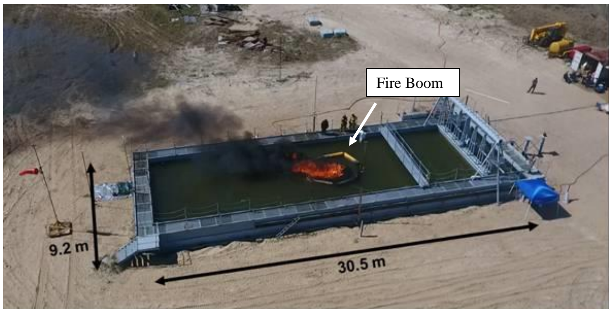
Figure 6. Overhead view of a burn with fire-resistant boom in place.
