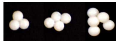
Fig. 10. ‘Granular Molecules’, each 3D-printed as one piece from hard plastic. Each sphere is \sim 3\text{mm} in diameter.
